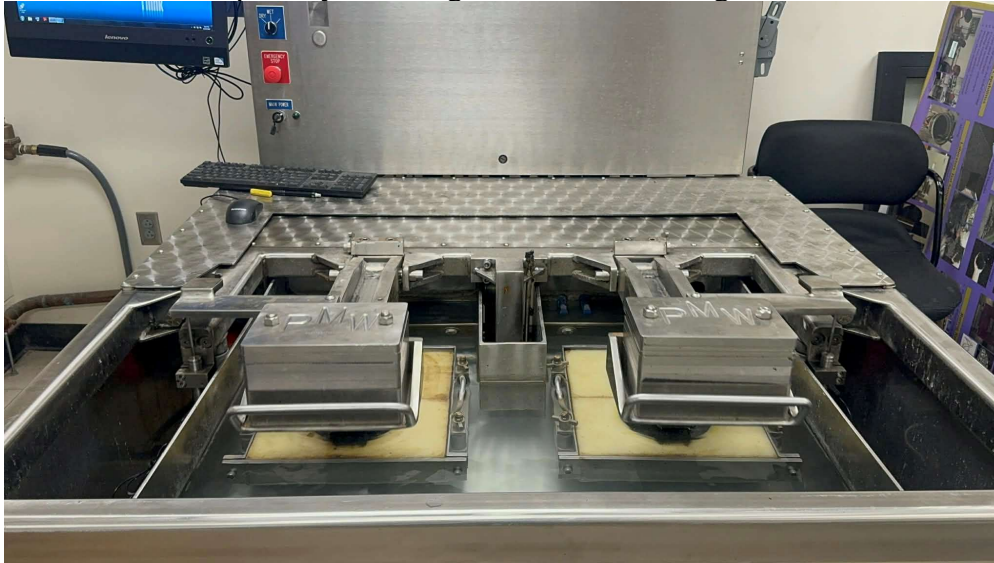
Figure 3.14: Hamburg wheel tracking device test setup
