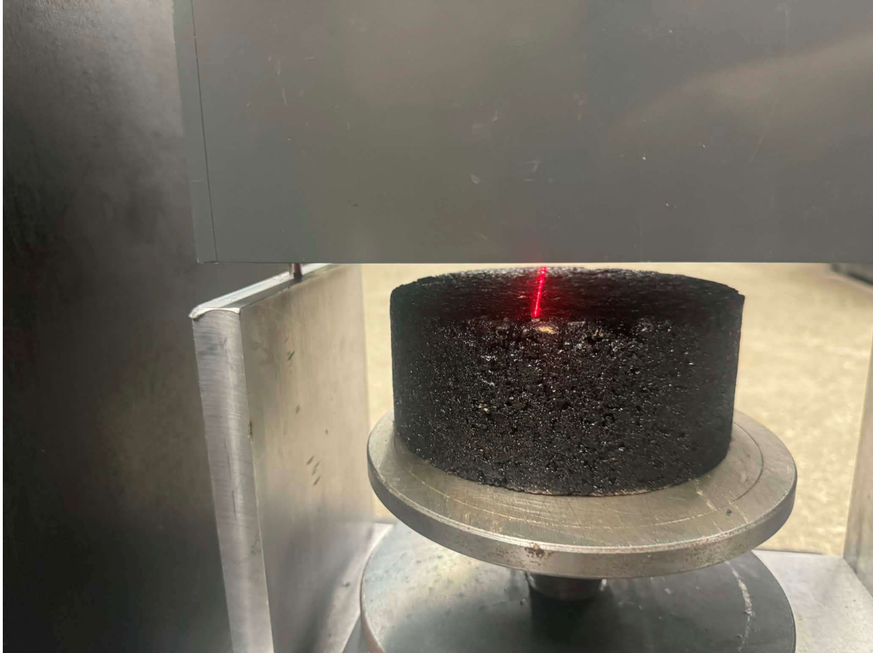
Figure 2.8: Sample setup in Laser Texture Scanner (LTS) showing the laser line scanning across the top surface of the asphalt specimen for macrotexture measurement.
