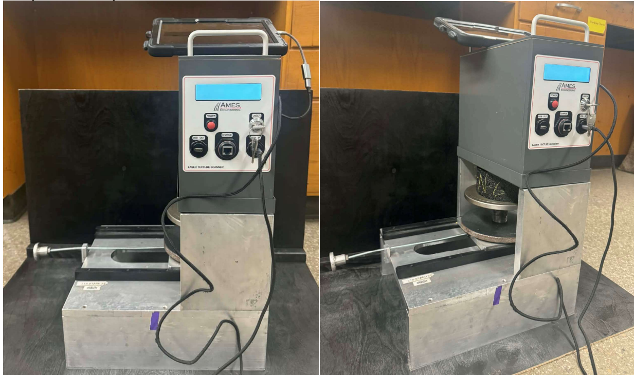
Figure 3.10: Laser Texture Scanner (LTS) test setup
