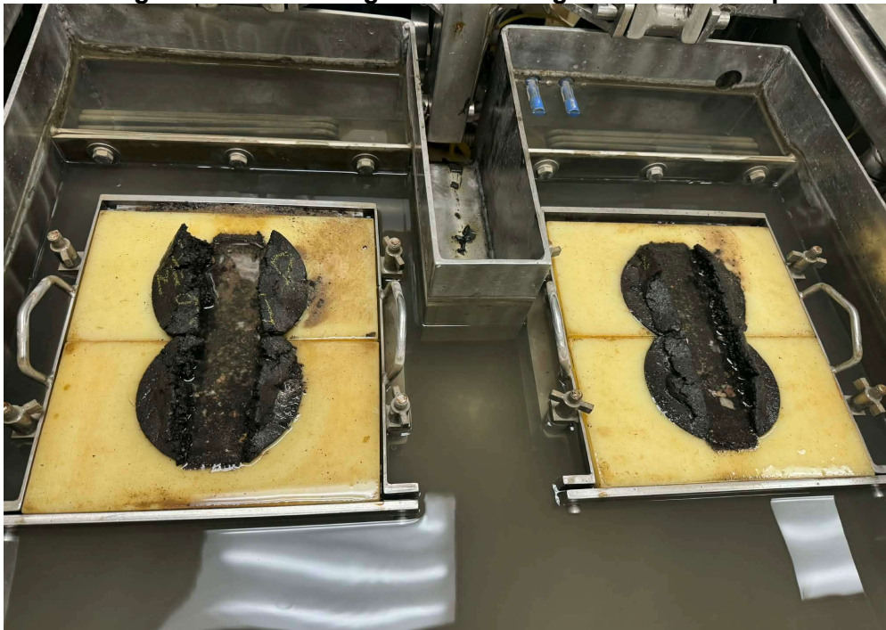
Figure 3.15: Specimens after completed HWTD test
