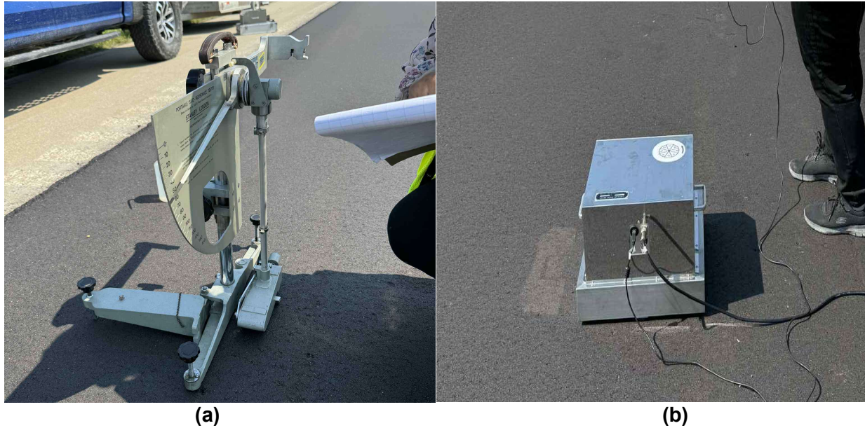
Figure 3.6: Field friction data collection (a) British Pendulum Test, (b) Circular Texture Meter (CTM)
