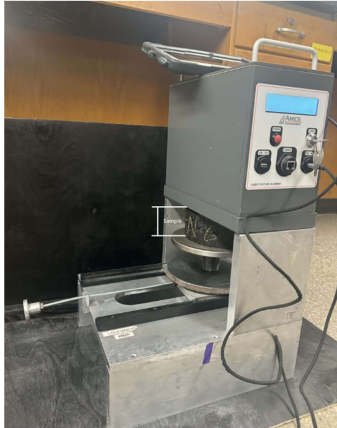
Figure 2.7: Sample setup in Laser Texture Scanner (LTS) for surface macrotexture measurement.
