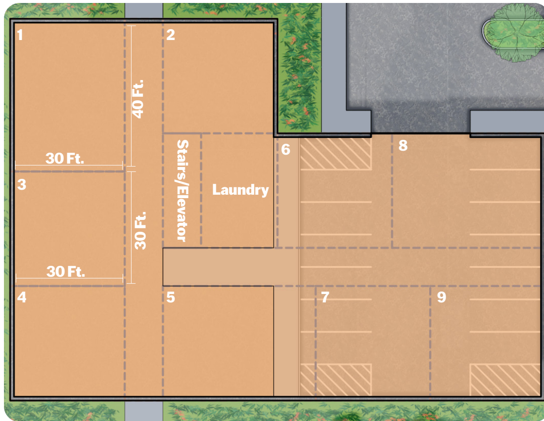
Figure 5.9 Layout of the Proposed Site 11 Structure (Saunders 2024). The proposed structure contains 41 1-bedroom units throughout 5 floors, a laundry room, and additional parking on the first floor.
