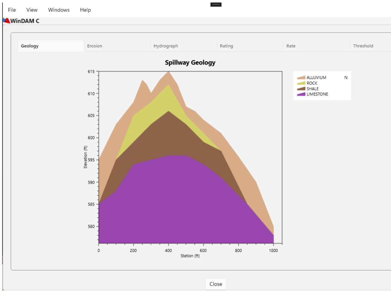
Figure 40. Summary Table - Aux. Spillway - View Geology Screen
