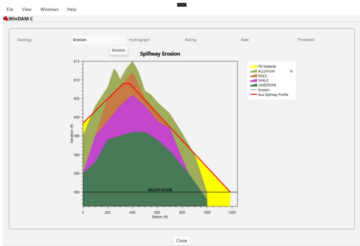
Figure 39. Summary Table – Aux. Spillway - View Erosion Screen
