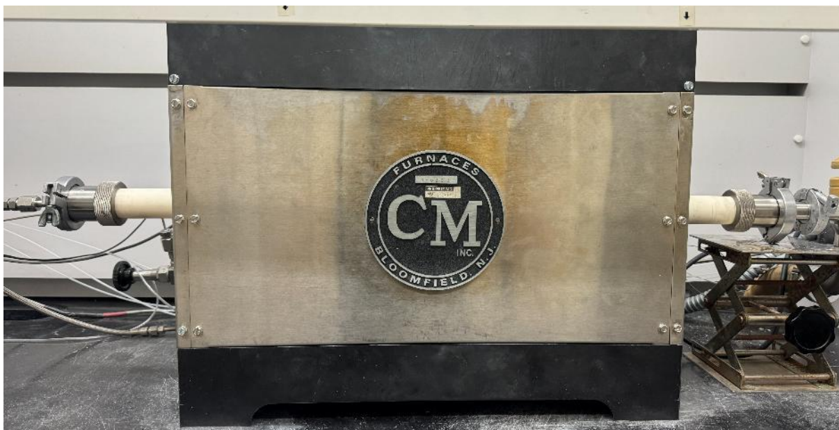
Figure 3.6. A closed horizontal alumina tube furnace with MoSi 2 resistive heating elements (not shown) used to grow hBN via APHT. Gas is supplied through the left side of the tube and flow is controlled using the valve on the right or a butterfly valve to regulate the pressure.
