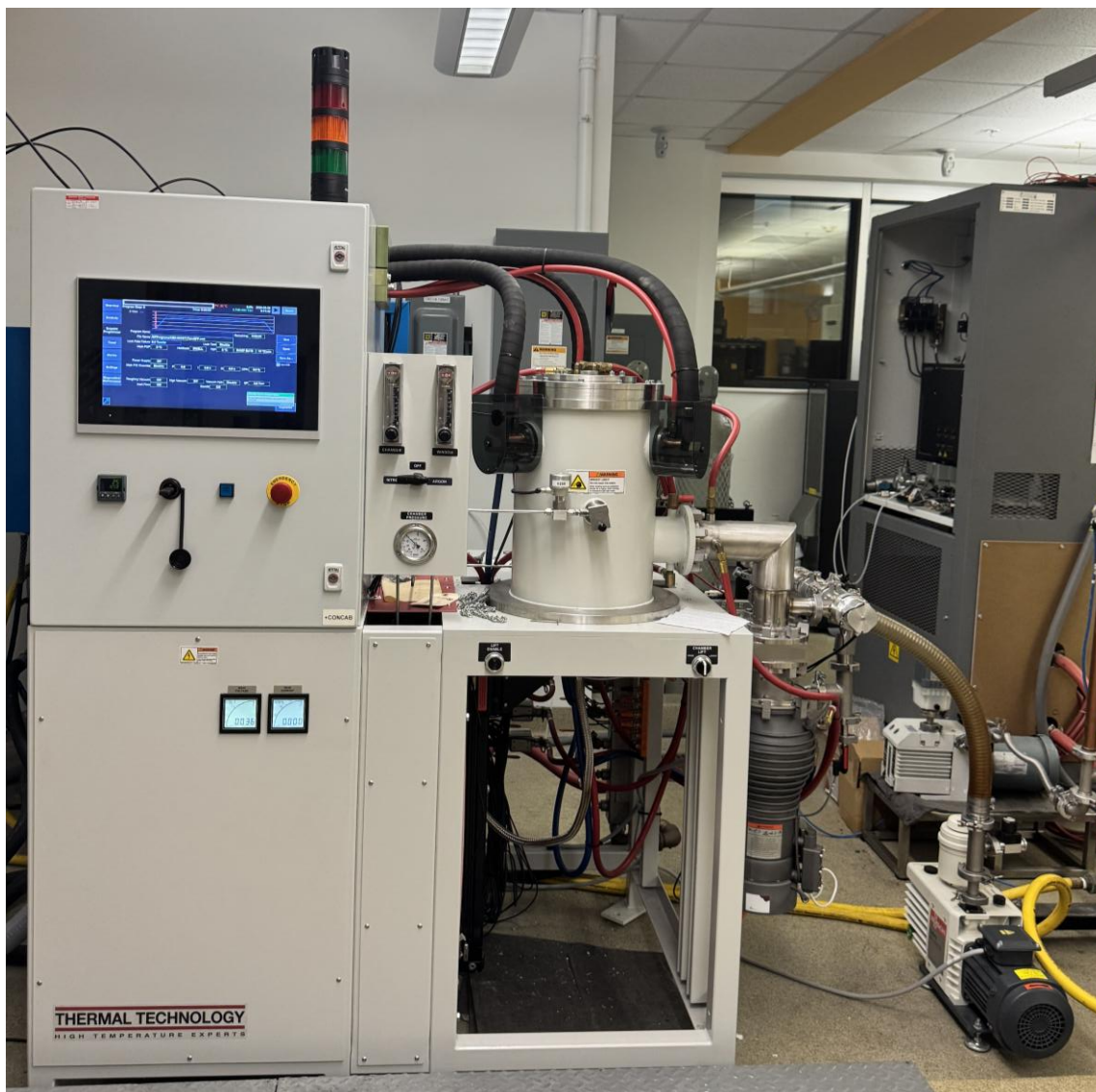
Figure 3.5 - Thermal Technologies Furnace equipped with tungsten heating elements and lined with stainless-steel heat shields
