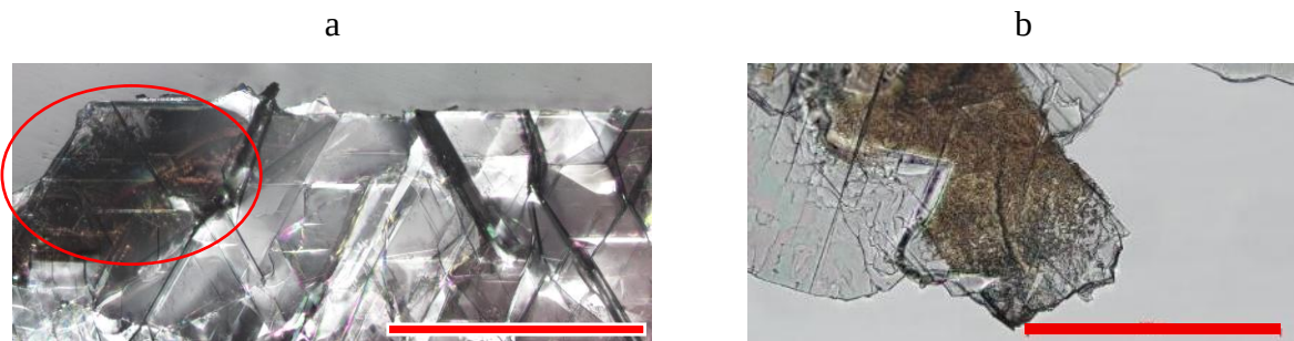
Figure 3.17 - Macroscopic defects caused by metal re-deposition on the hBN crystal in (a) reflection and (b) transmission. Scale bar is (a) 1000 \mu\text{m} and (b) 500 \mu\text{m} .
