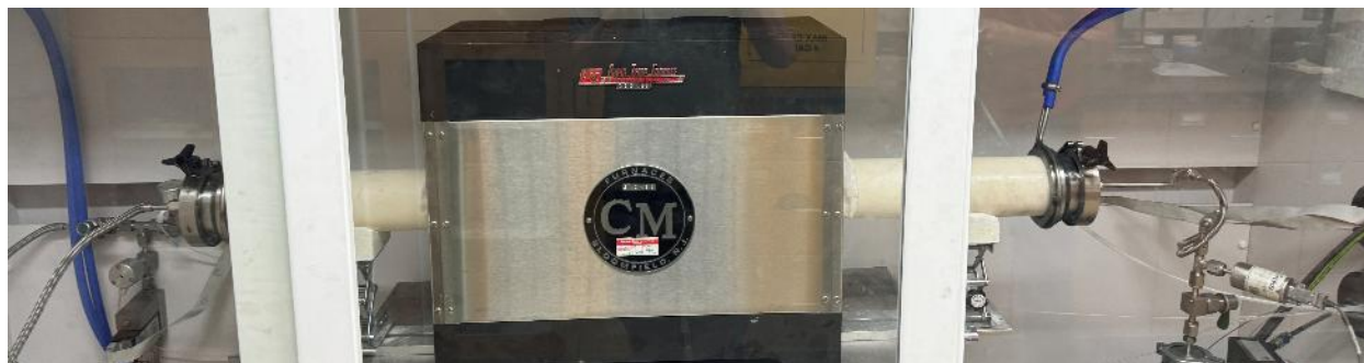
Figure 3.8 - Image of LCM apparatus. Gas is supplied from the left and pumped out on the right. Pure hydrogen was available for this furnace as opposed to forming gas.
