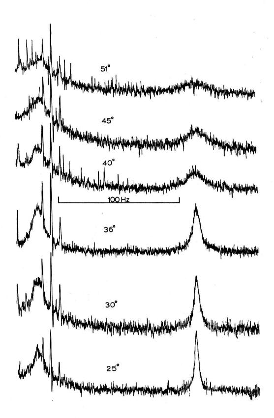
for methyl group exchange between methyllithium and dimethylmercury was obtained from measurements of the methyllithium linewidth at various temperatures. A  $1/ au_{
