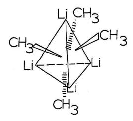
McKeever, et al. (4), have verified this tetramer structure by noting  $^7\text{Li-}^{13}\text{C}$  scalar coupling in the  $^7\text{Li}$  magnetic resonance spectrum. However, Brown, et al. (5), have noted that the metalmetal bond order between lithium atoms may be zero, due to the absence of observable  $^7\text{Li-}^6\text{Li}$  scalar spin-spin coupling at low temperature.
