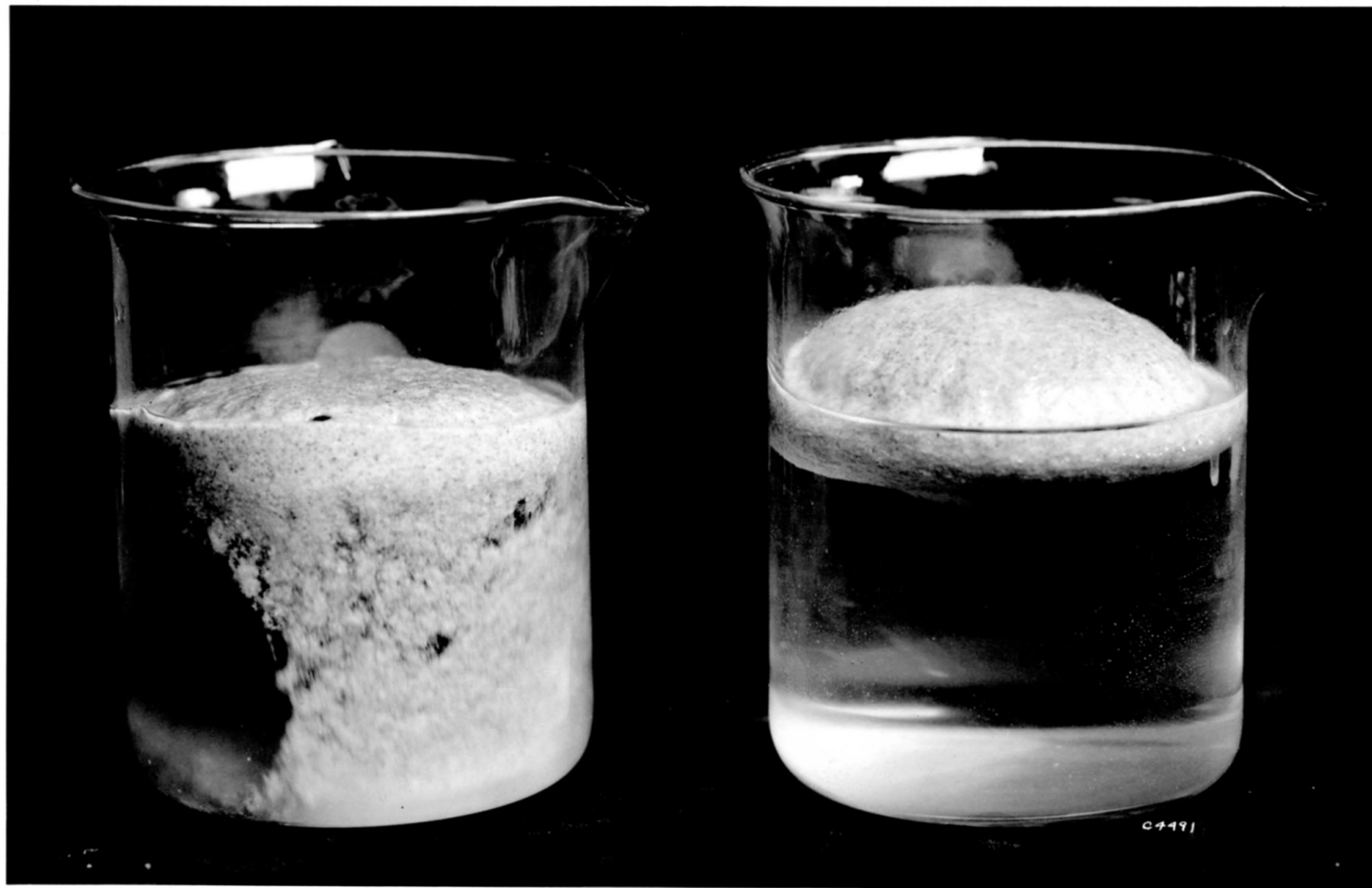
Doughballs in wheat meal fermentation time test of Blackhull (left) and Tenmarq (right). Breaking "time" for Blackhull, 51 minutes, and for Tenmarq, 102 minutes.
