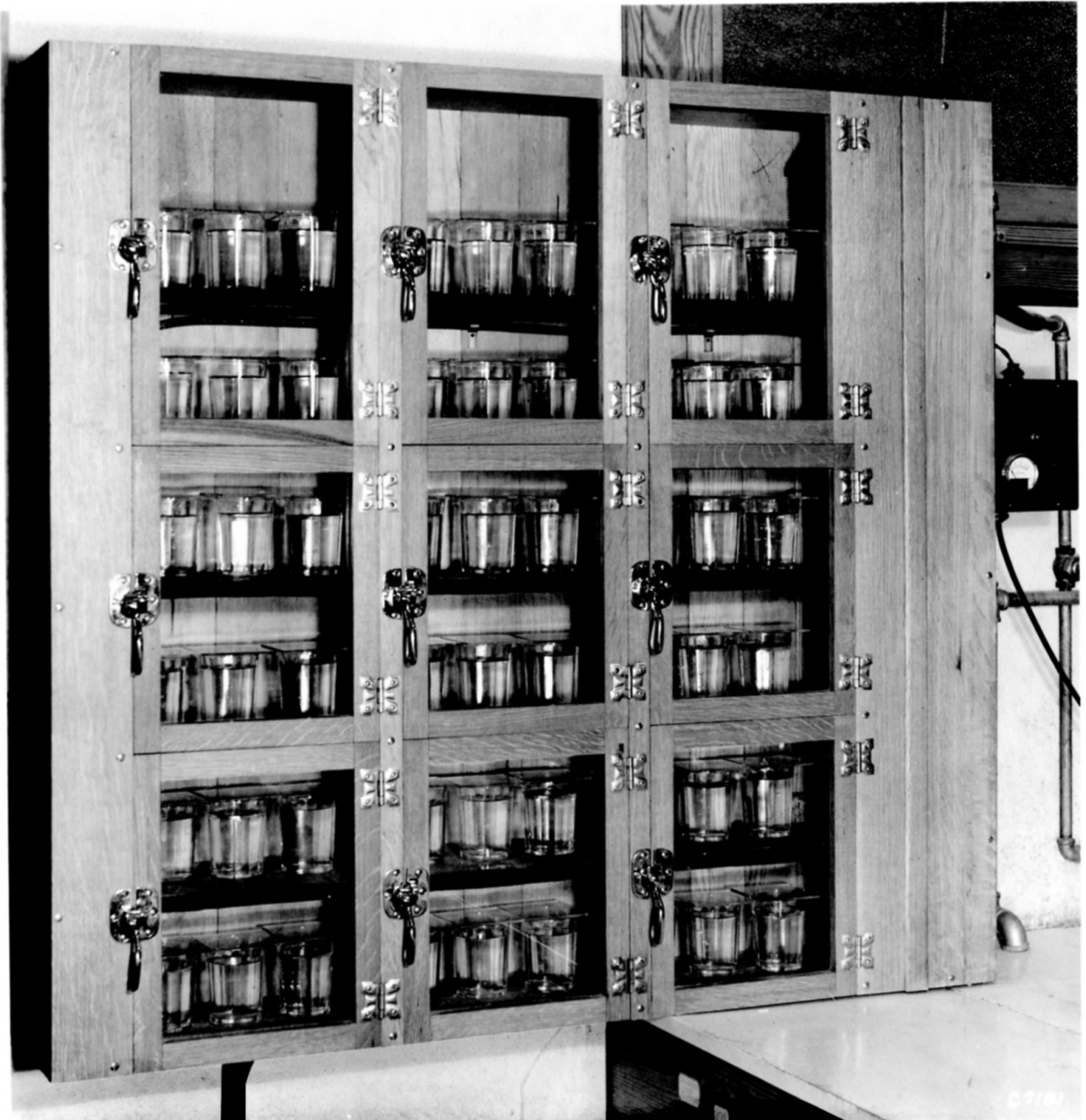
Temperature controlled cabinet, designed in the Department of Milling Industry, Kansas State College, for maintaining constant temperatures while "time testing" samples.
