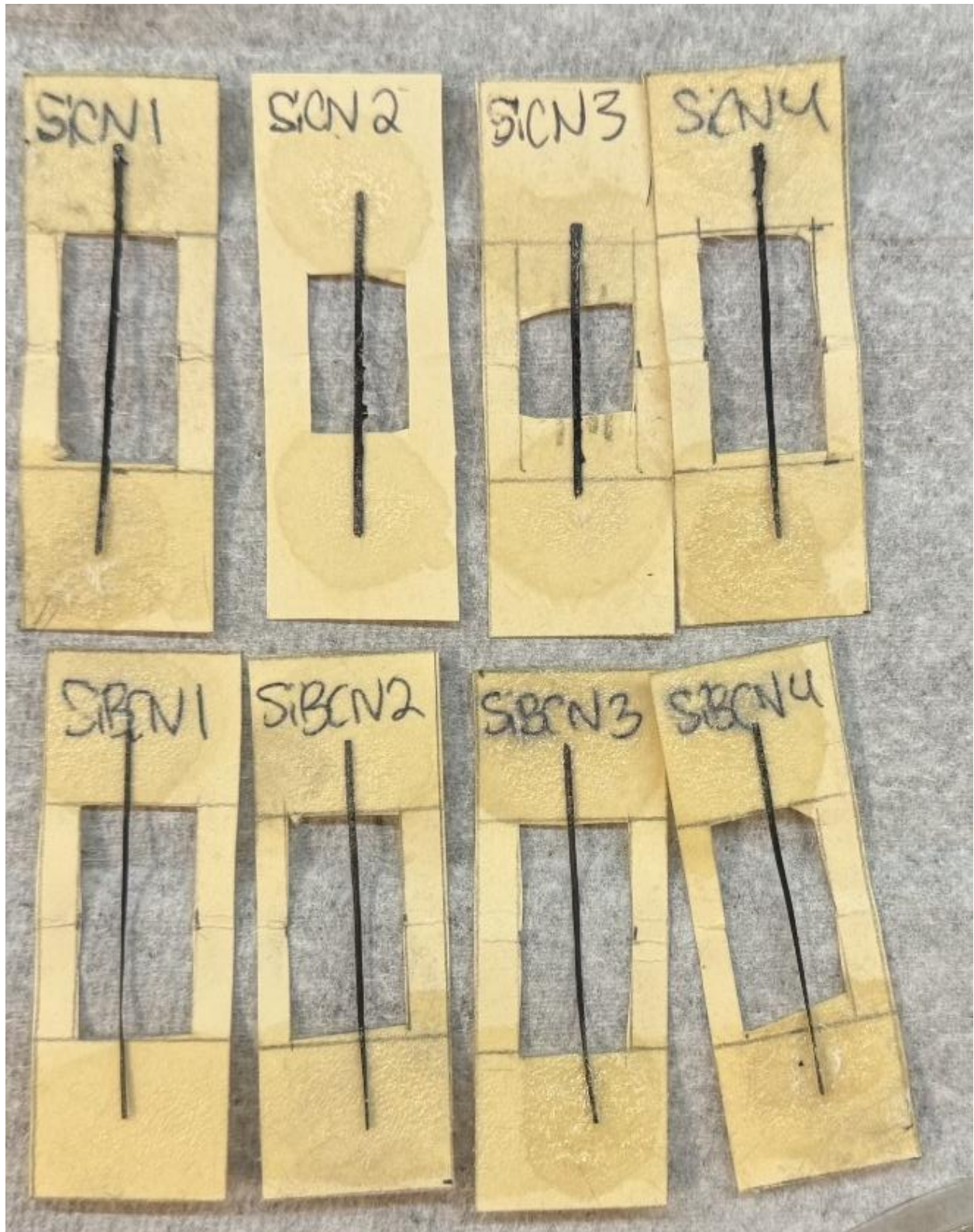
Figure 3-10: Tensile Test Samples with Applied Glue to Mounts
