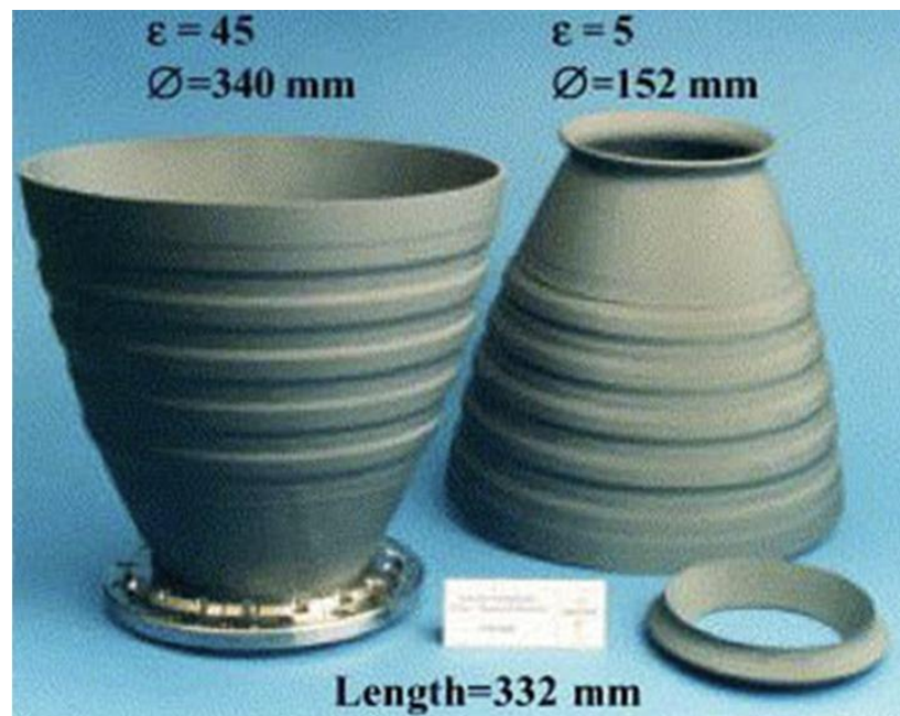
Figure 1-10: C/SiC Nozzle Extensions developed for ULA's Vulcan Cryogenic Engine [10]
