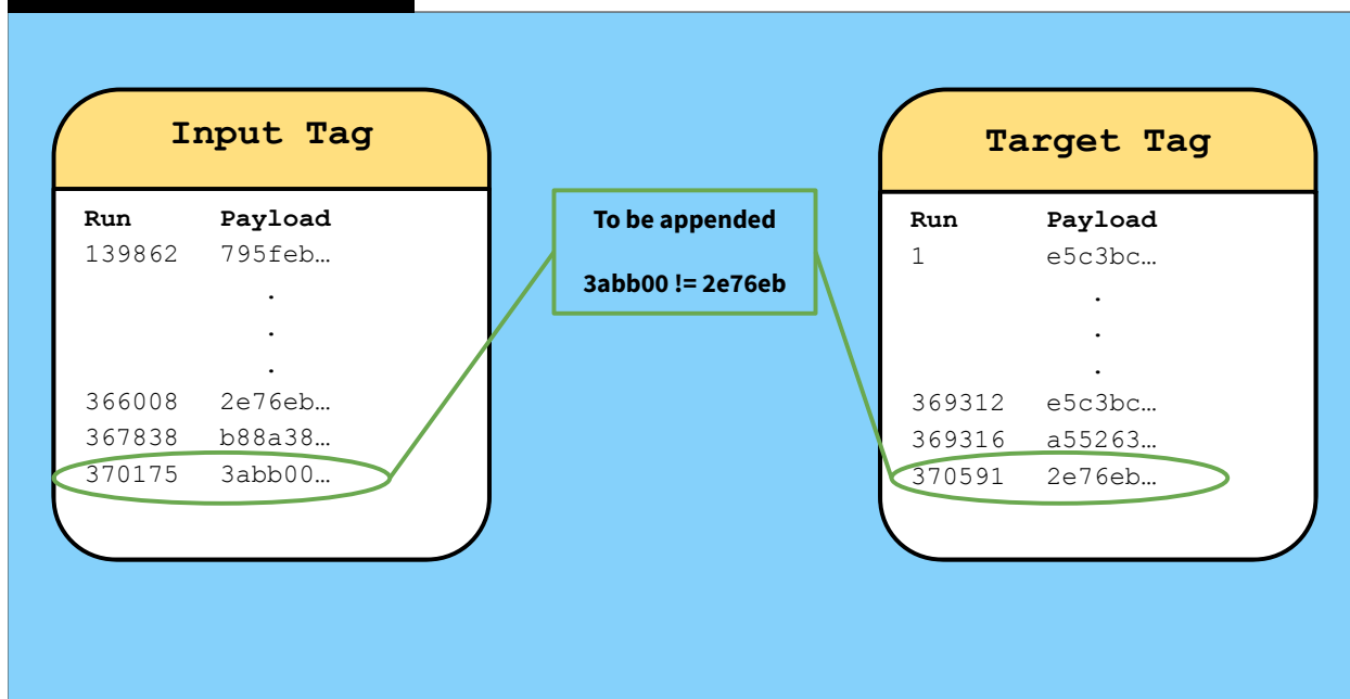
Figure 4.5: An example of the appending procedure in O2O. In this example, the most recent payload on the input tag (left) will be appended to the target tag (right) because they are not the same.
