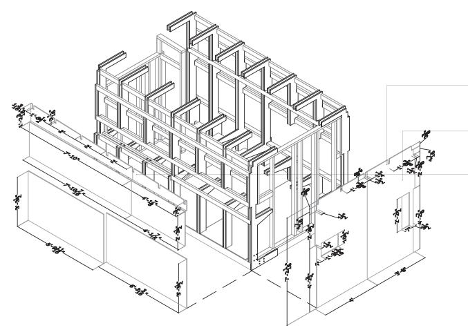
**STEP 6** Exterior osb attachment—front & left sides
