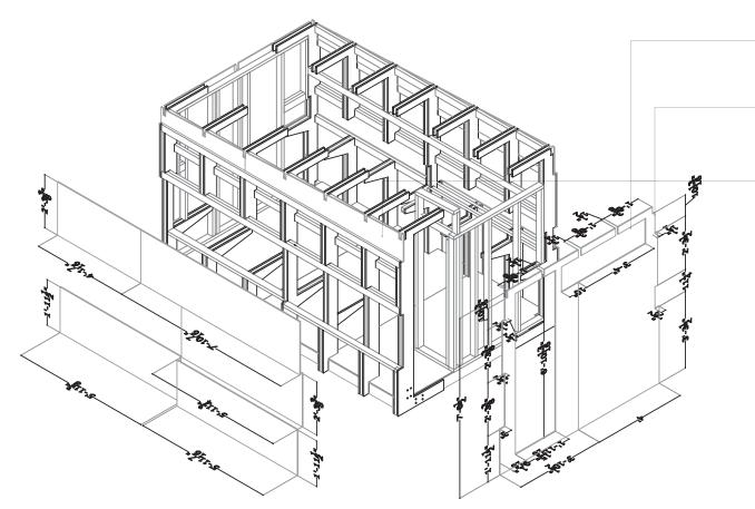
**STEP 6A** Exterior osb attachment—back & right sides
