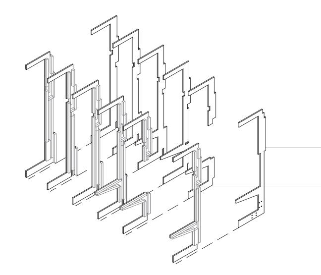
**STEP 2A** Plywood composite structure sub-assembly—right side
