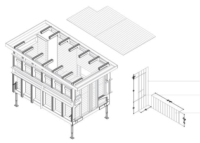
**STEP 10** Interior bamboo attachment Front and sliding door attachment
