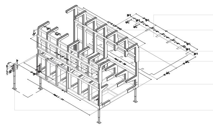
**STEP 3** Jack attachment, install header, subfloor, & structure
