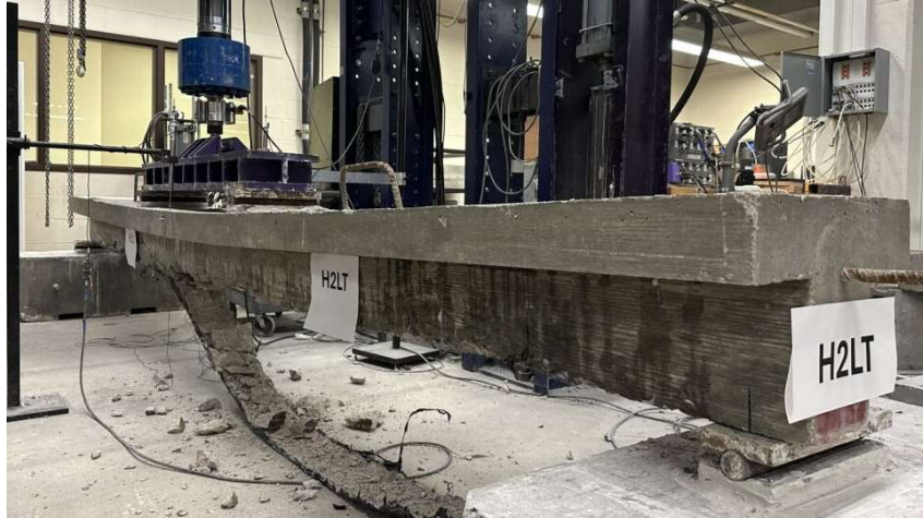
Figure 4.39: H2LT beam after testing
