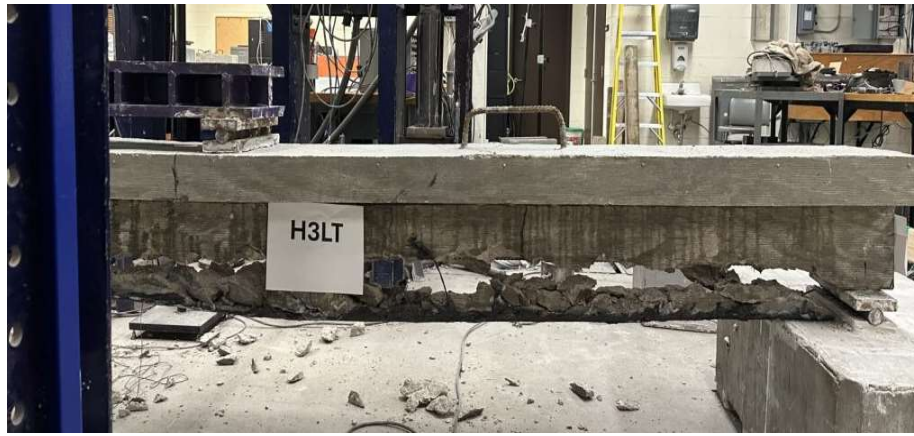
Figure 4.44: H3LT beam after testing
