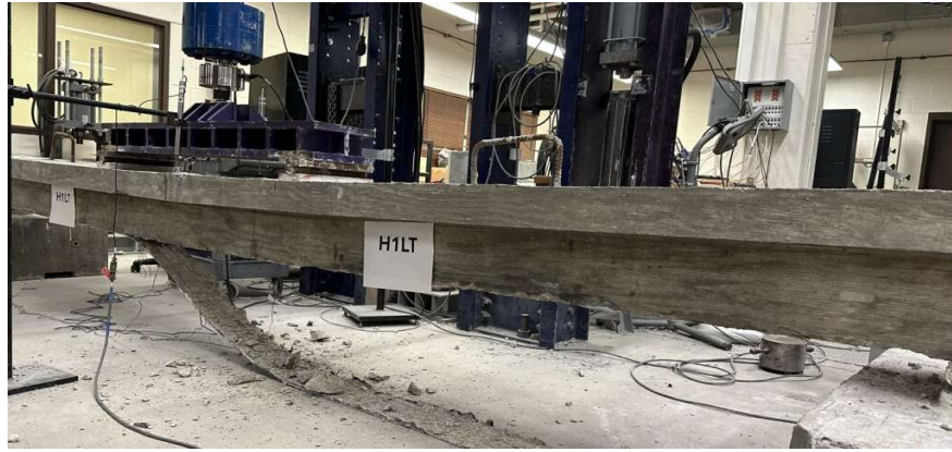
Figure 4.34: H1LT beam after testing
