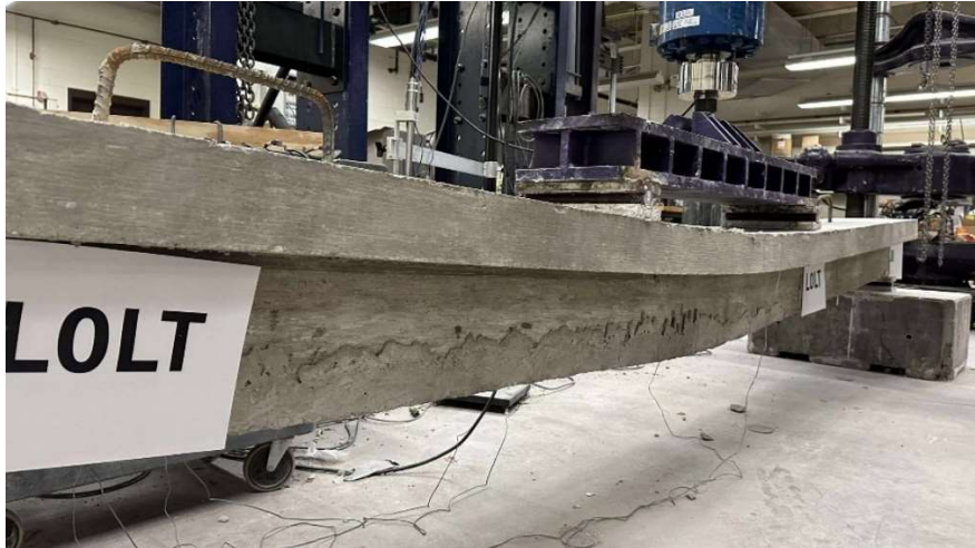
Figure 4.5: LOLT beam after testing
