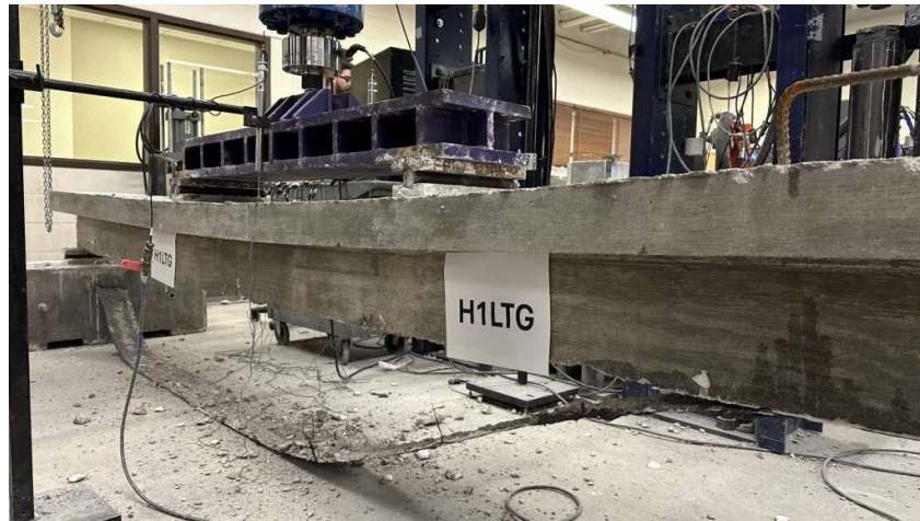
Figure 4.49: H1LT beam after testing
