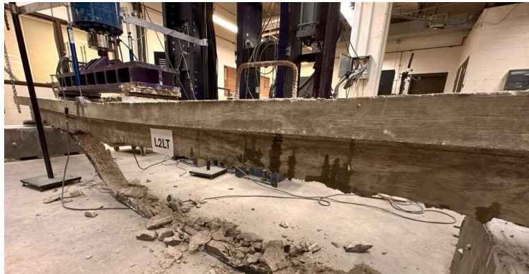
Figure 4.14: L2LT beam after testing
