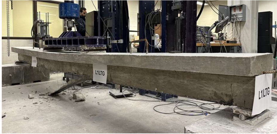
Figure 4.24: L1LTG beam after testing
