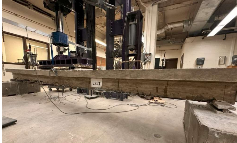
Figure 4.19: L3LT beam after testing
