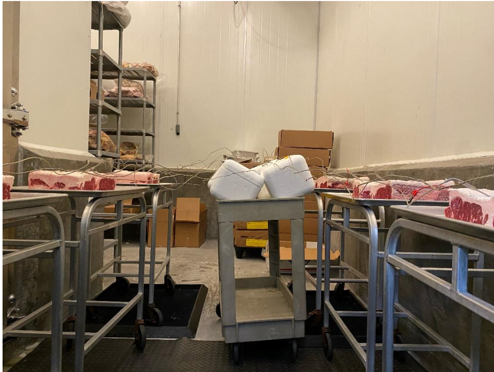
Figure 2.1: Representative image of EM treatment set up with temperature probes
