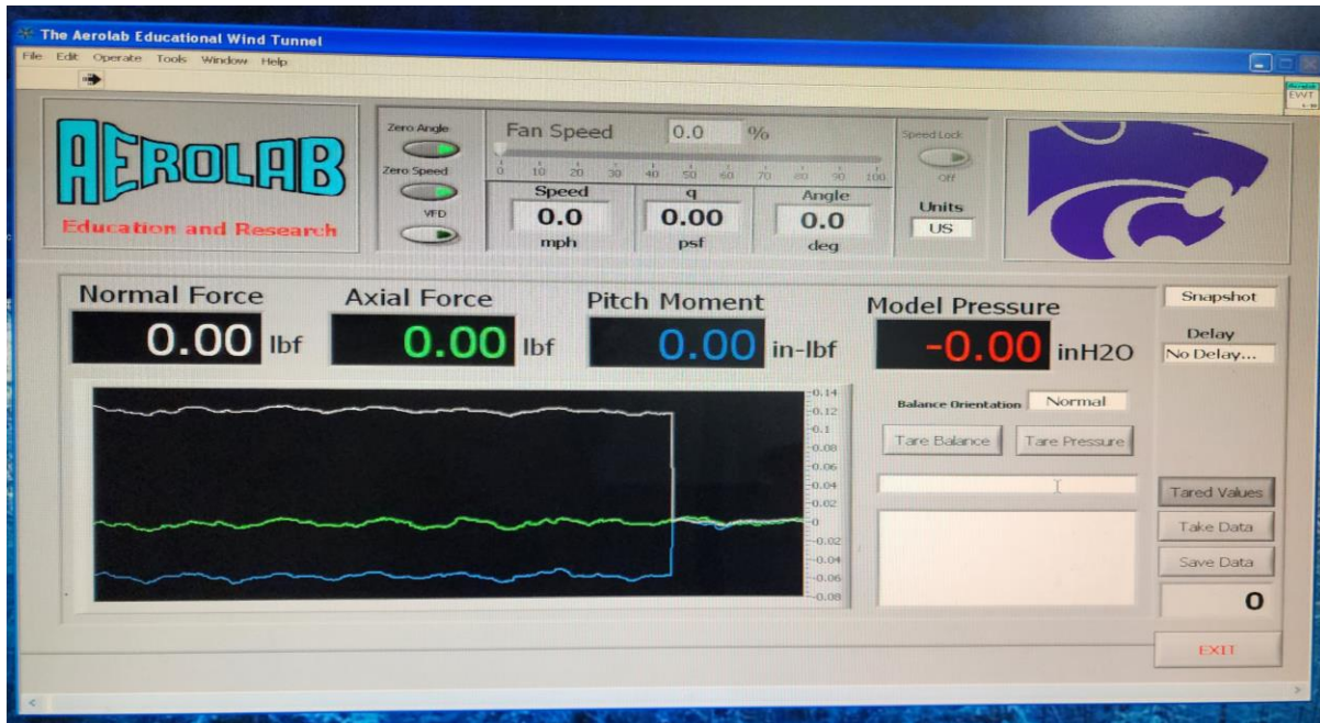
Figure 3.5 – AEROLAB LabVIEW User Interface
