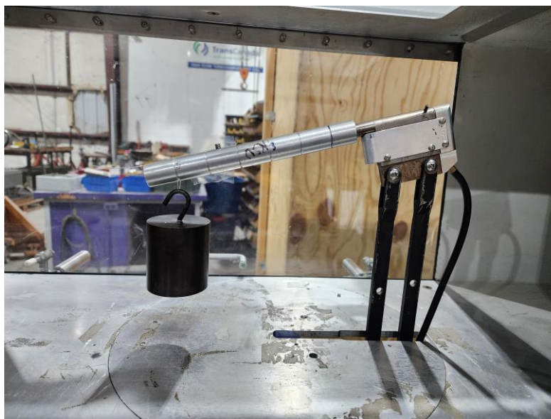
Figure 3.11 - Sting Balance Calibration Set-Up
