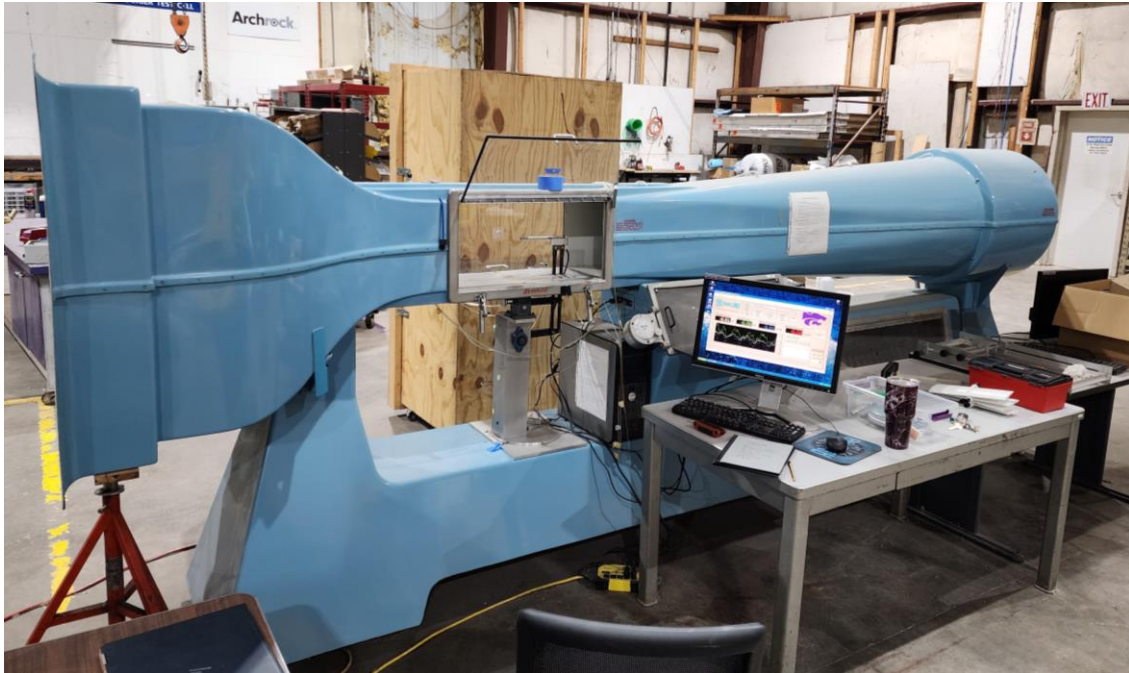
Figure 3.2 – AEROLAB Wind Tunnel
