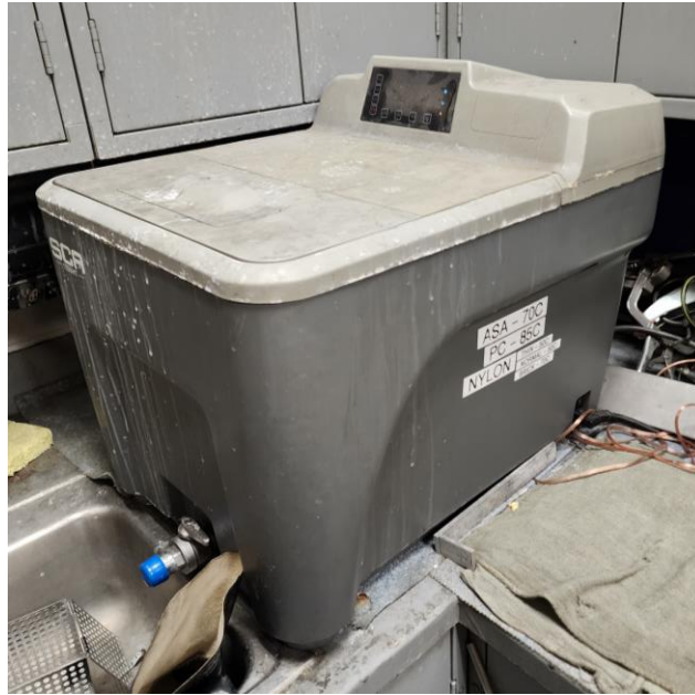
Figure 2.21 - Support Removal Apparatus
