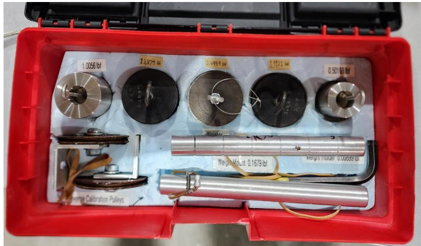
Figure 3.9 - Calibration Weights & Sleeve
