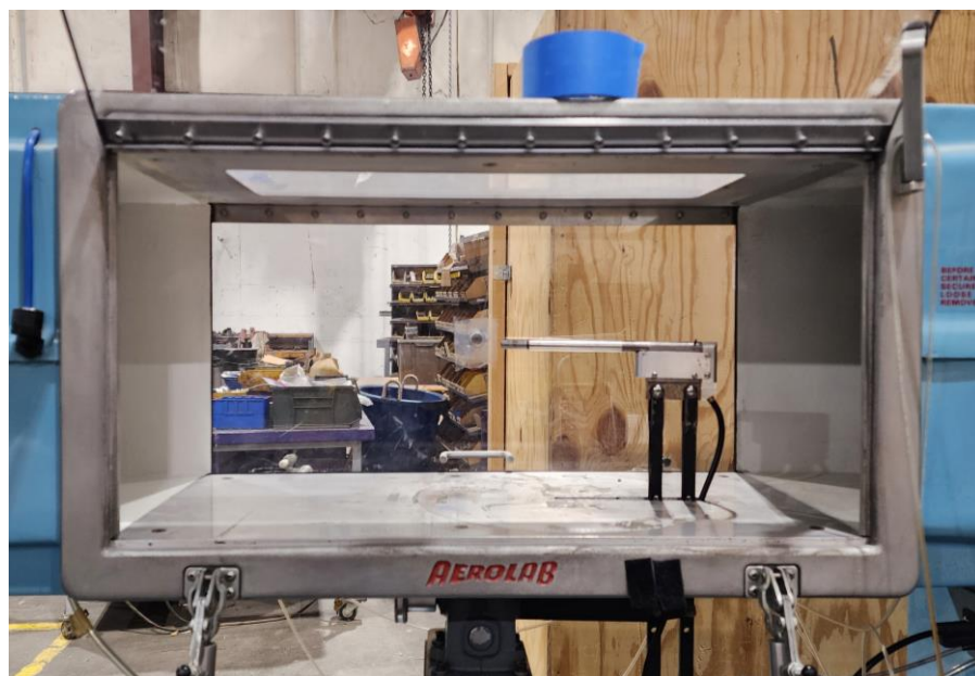
Figure 3.3 - Wind Tunnel Testing Section and Sting
