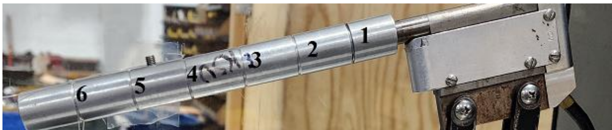
Figure 3.10 - Sting Balance Sleeve with Positions Marked
