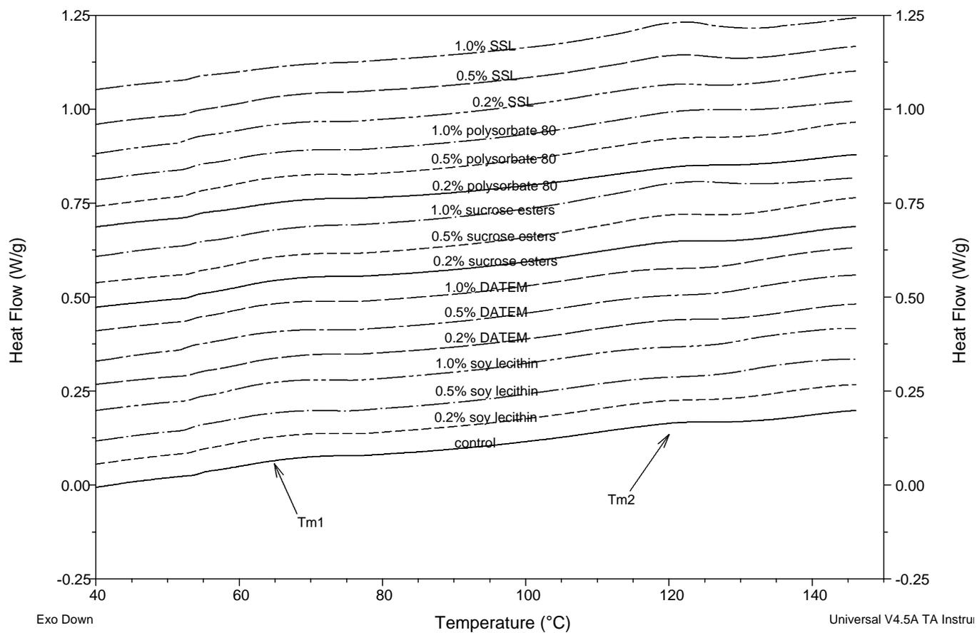
**Figure 5.8** DSC thermograms of whole wheat bread with added emulsifiers stored for 7 days
