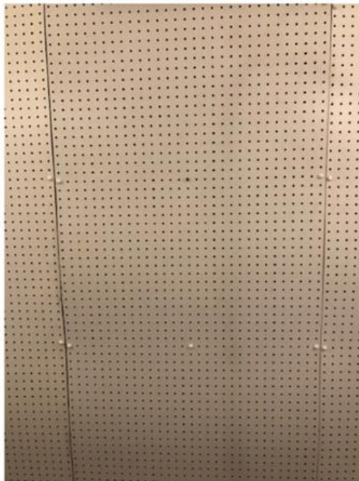
Figure 3.6 Inlet velocity wall.
