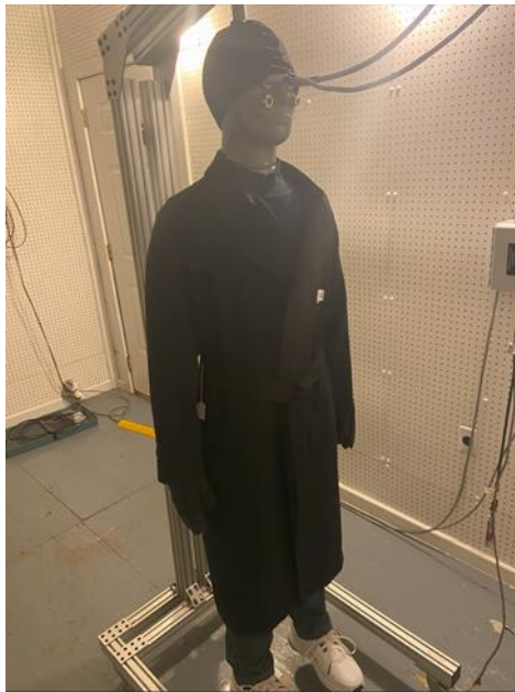
Figure 3.4 Thermal manikin in climactic chamber.
