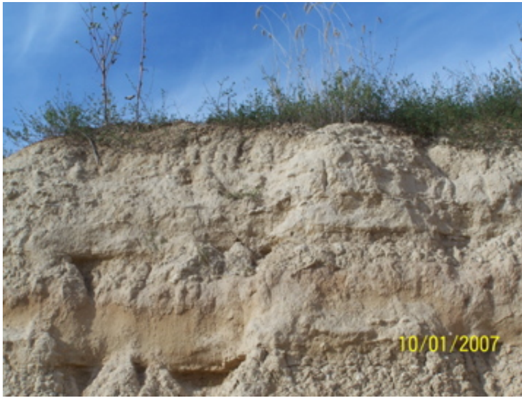
Figure A2.19. KS-45B located in McPherson County, KS. Tephra sample is mixed with a significant amount of silt. Laboratory procedures yielded insignificant amount of tephra.
