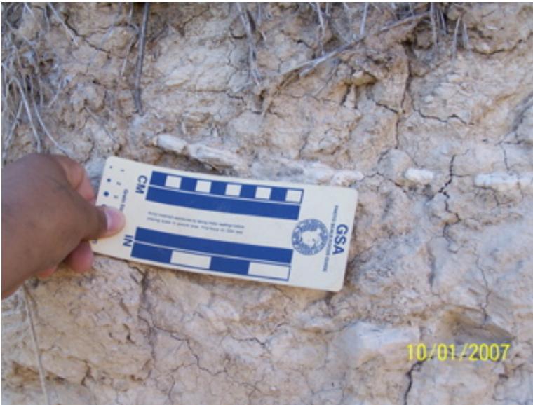
Figure A2.18. KS-45A located in McPherson County, KS. Outcrop consisted of small gravel size impure-tephra clasts interbedded with silt. Could not isolate significant tephra during laboratory procedures.
