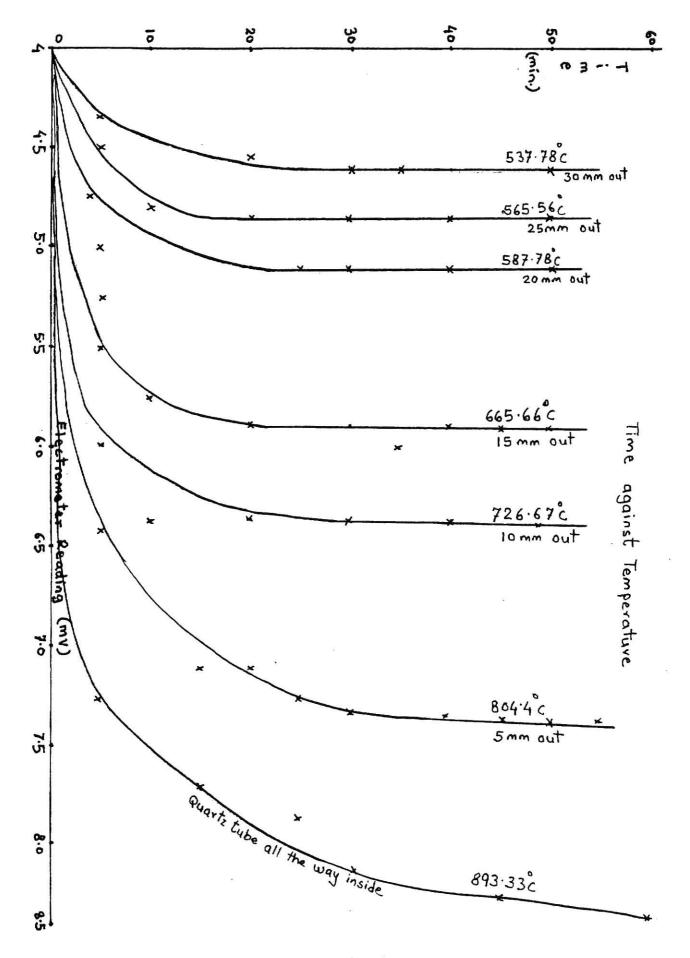
Figure 5. Temperature as a Function of Position of the Quartz Tube.
