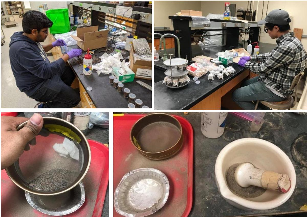
**Figure 3.14.** Soil laboratory activities (indoor portion)—preparing soil samples for PLFA analysis. (Images taken by M. M. Lekhon Alam and James Lin on October 10, 2019, at the Department of Agronomy, KSU.)
