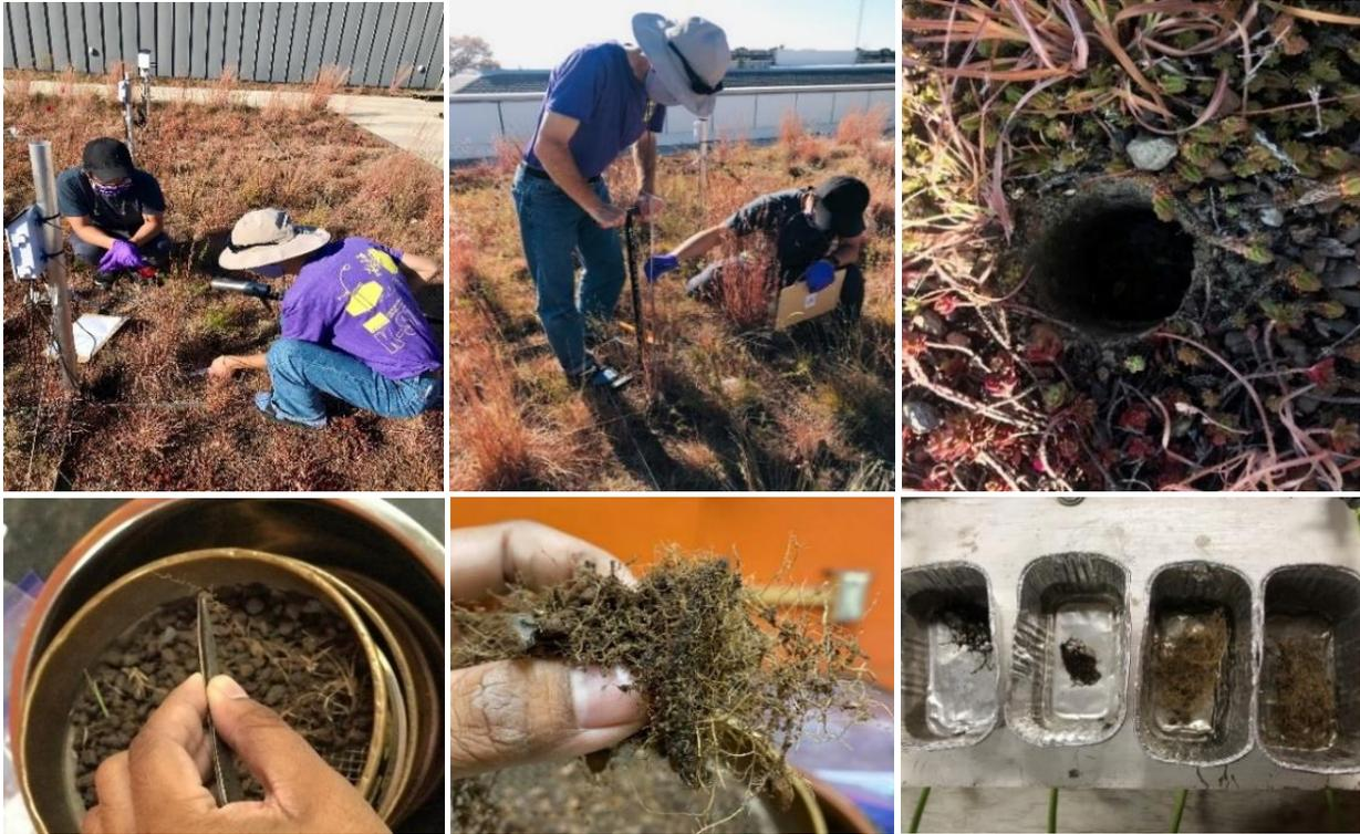
**Figure 3.13.** Collecting and analyzing root biomass samples from the 4-inch-/10-cm- and 8-inch-/20-cm-deep beds. (Images taken by M. M. Lekhon Alam on November 6, 2020.)
