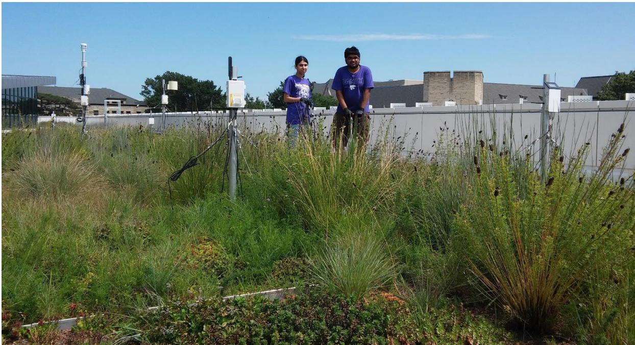
**Figure 3.12.** Collecting soil samples for respiration analysis from the APD-EGR's 4- and 8-in-deep beds in 2020 (outdoor portion).
