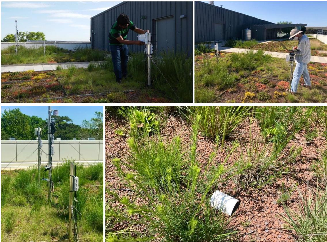
**Figure 3.17.** Installing temperature sensors, checking sensor readings, and an assortment of temperature and soil moisture sensors at APD-EGR
