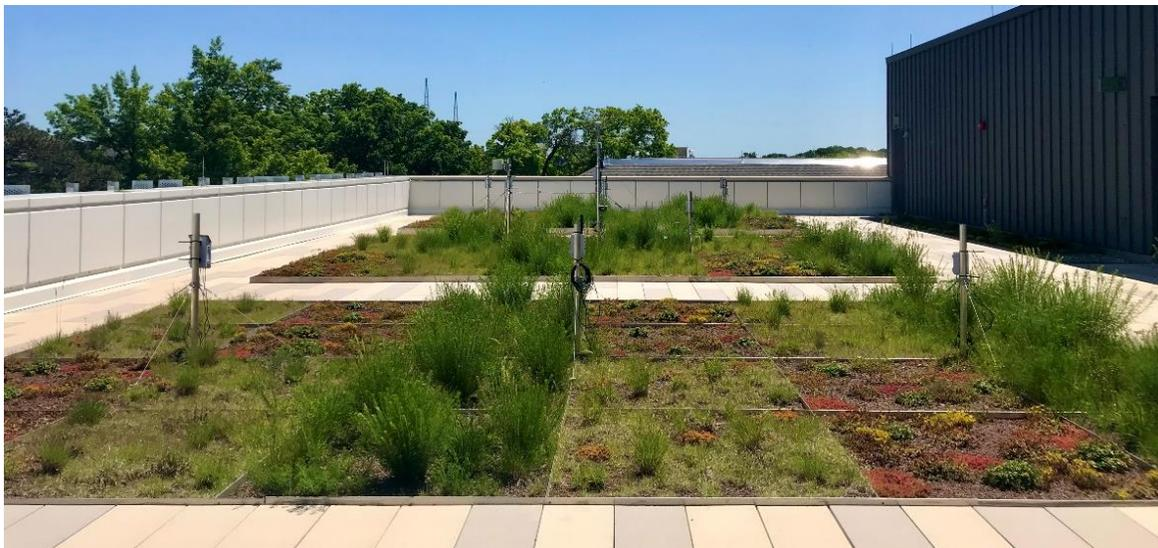
**Figure 1.2.** Photo of the APD-EGR at KSU showing the 4-, 6-, and 8-inch deep APD-EGR beds (the 4-inch bed is closest to the camera).
