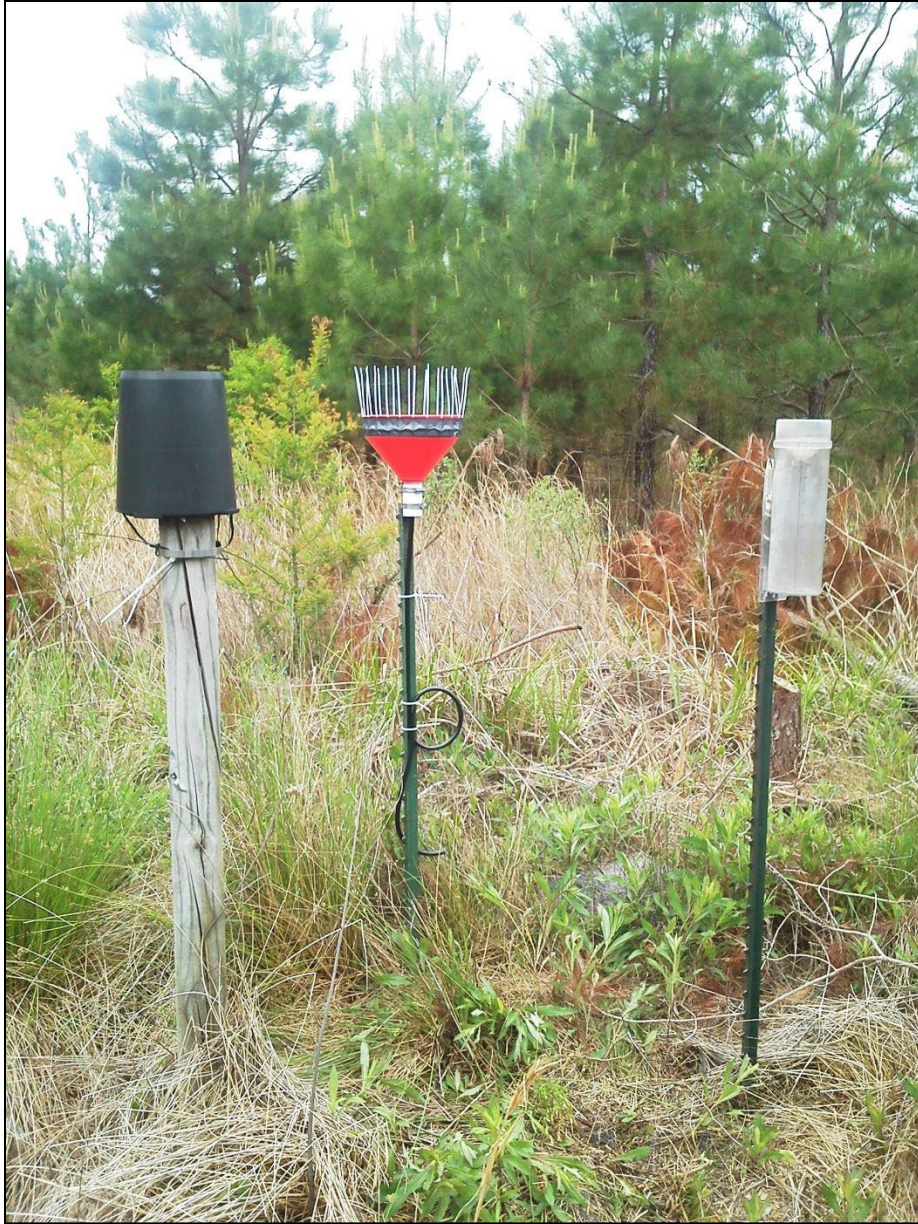
SI Figure 5. The apparatus used for collection of atmospheric deposition of P, alongside a tipping bucket rain gauge and a traditional rain gauge. The sample collection bottle is not shown.
