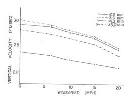
they entered the airstream due to the Bernoulli effect. Static pressure was found to be greater in the wind tunnel than in the still air above the tunnel. Therefore, the drops were falling from a lower to higher pressure area. The decrease in vertical velocity was probably due to both lift and pressure gradient.
