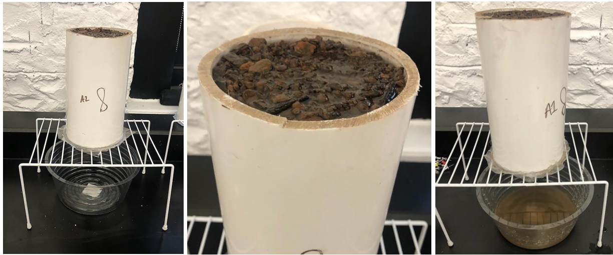
Figure 3.1. Pictures (from left to right) Show the PVC Setup with Rack and Bucket Beneath, Thin Layer of Water at Surface of Substrate after Saturating, and a PVC Column Draining.
