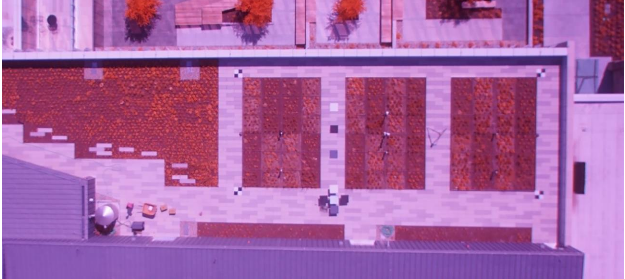
Figure 1.3. Aerial Photo of the APD Experimental Green Roof. Small unmanned aerial vehicle (sUAV) infrared image taken July 18, 2018 by Harman Singh, showing the live plant planting pattern within each cell and the two different substrate types in four distinct blocks in each bed or area.
