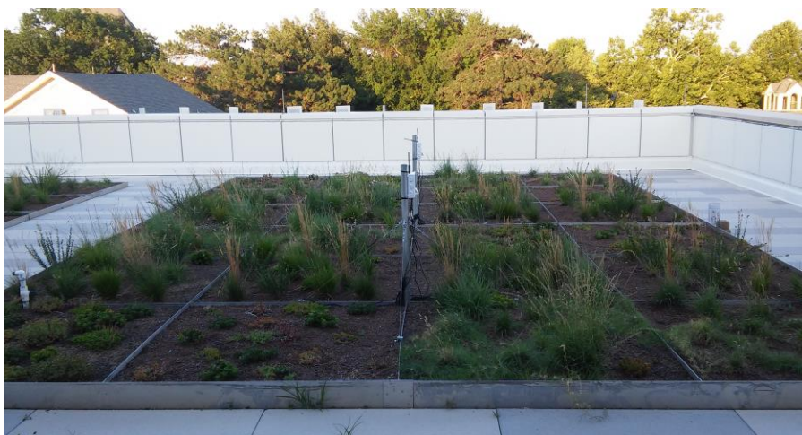
Figure 1.4. Photos of the APD-EGR. Photos a, b, and c of the three planting areas—the 4-inch bed, 6-inch bed, and 8-inch bed (respectively), taken July 19, 2018 by Lee Skabelund (looking east at the three planting areas). Data-loggers attached to metal poles are connected to various sensors.
