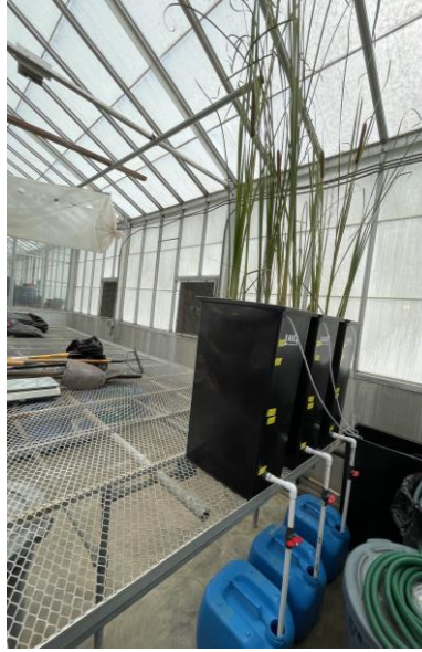
Figure 5.1. VFCWs systems set-up.
