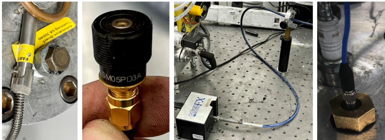
**Figure 2.4:** *From left to right: temperature probe, photodiode, spectrometer with fiber optic, and piezocrystal.*
