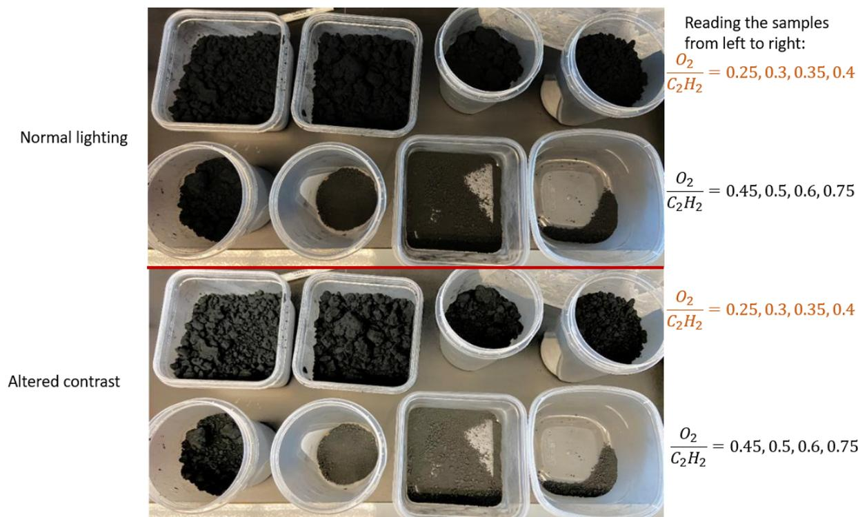
**Figure 3.9:** *iPhone SE picture of graphene samples. The top picture is captured in normal room lighting, and the bottom picture has altered contrast for visibility purposes. A thin red line is drawn between the pictures for clarity. The four samples in the top row are the 0.25, 0.3, 0.35, and 0.4 O/C, and in the bottom row 0.45, 0.5, 0.6, and 0.75 O/C.*
