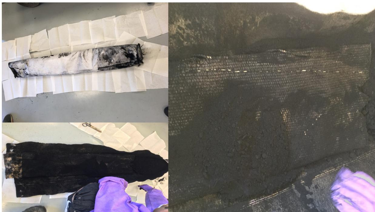
**Figure 4.2:** *Top left: bag filter after collecting 1 kg of graphene. Bottom left: graphene-coated Kevlar on the inside of the cut-open bag filter after collecting 1 kg of graphene. Right: close-up picture with altered contrast of the Kevlar and cut-open bag filter.*
