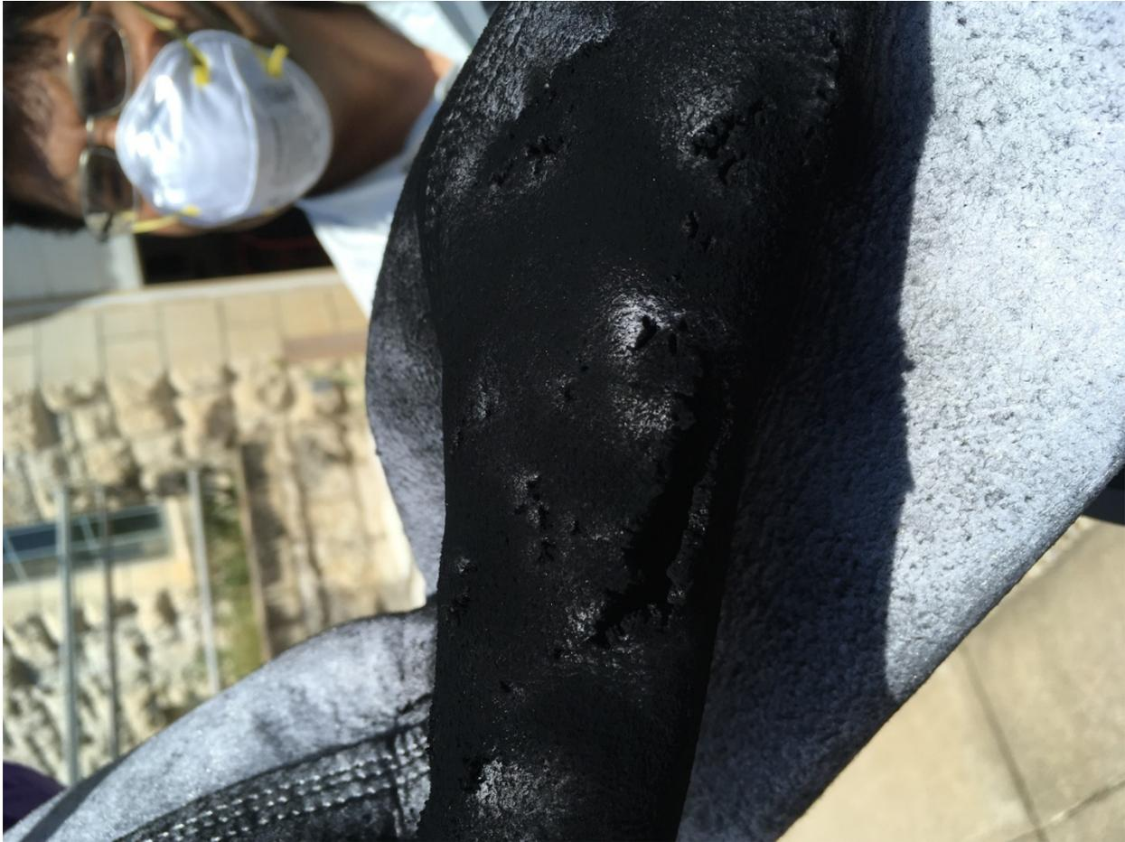
**Figure 4.6:** *Picture of holes burned through the top half of silicon bag filter. The face of Dr. Arjun Nepal is seen in the background.*
