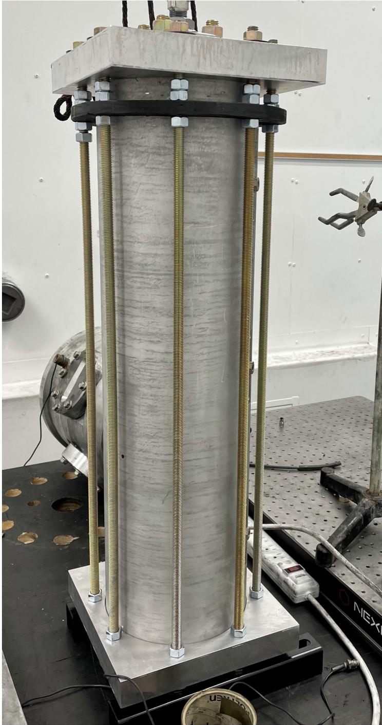
**Figure 5.23:** *Newly constructed 17 L skinny detonation chamber.*
