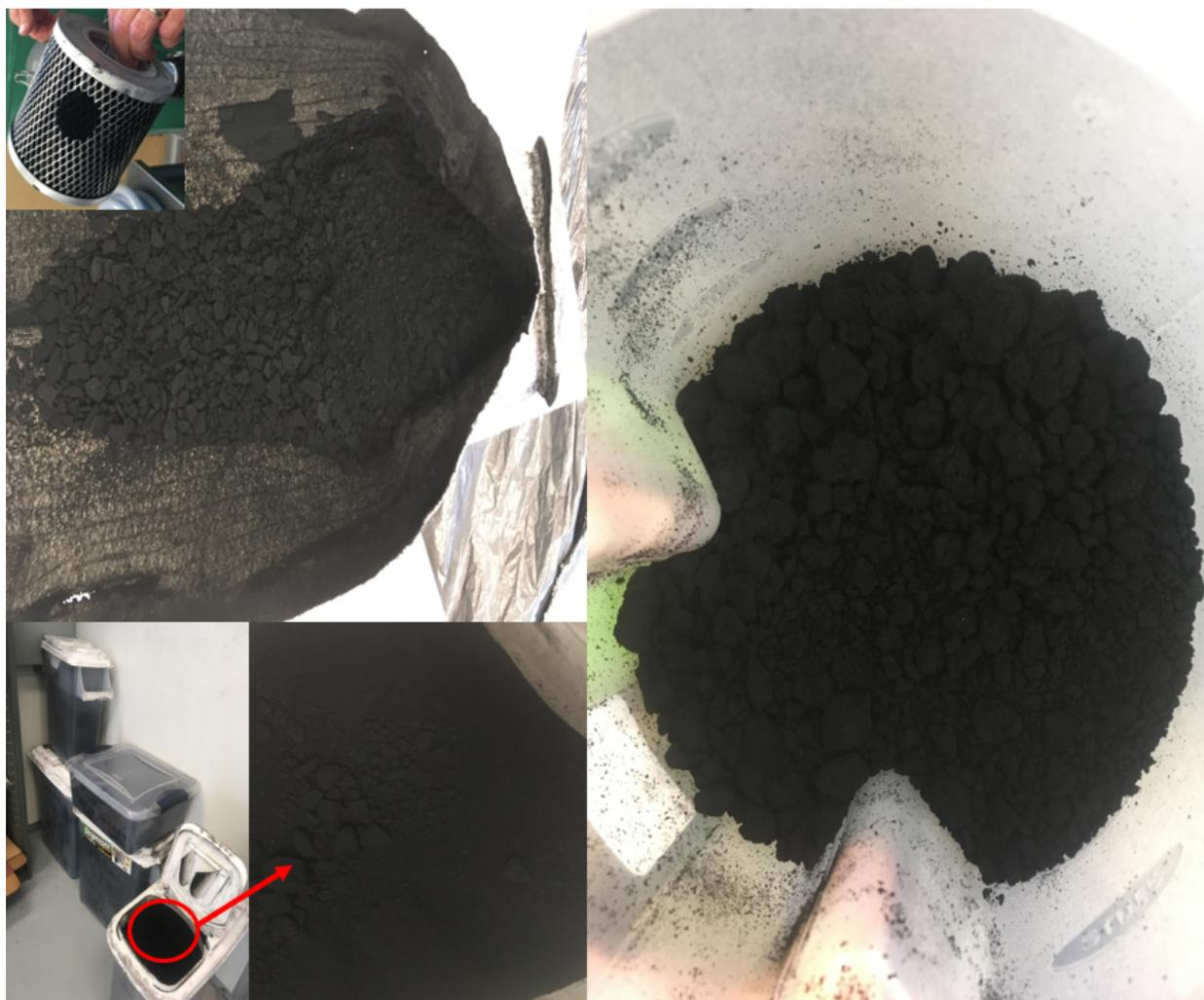
**Figure 4.5:** *Top left: bag filter cut open to reveal graphene inside and picture of HEPA filter; bottom left: 10 kg of graphene collected and stored with a closeup image of the sample; right: single shot graphene sample from the 17 L chamber for comparison.*
