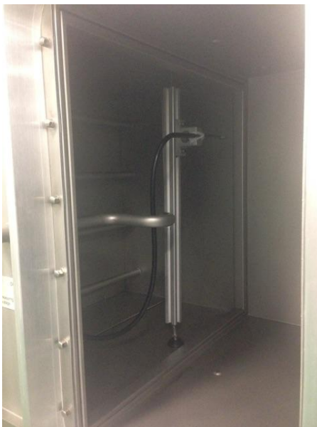
Appendix Figure A.2. Our testing device for Aerosol distribution upstream & downstream filter
