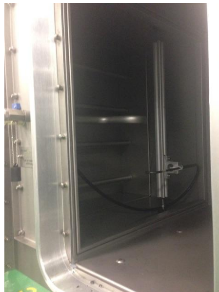
Appendix Figure A.2. Our testing device for Aerosol distribution upstream & downstream filter
