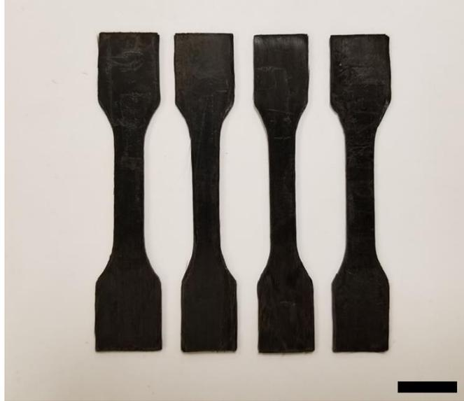
**Figure 4-4** Some of the tensile bars used for tensile testing (scale bar: 14 mm).
