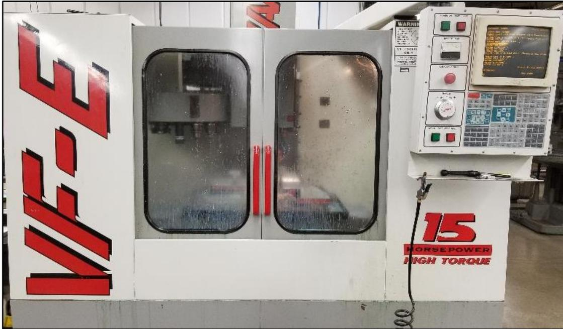
**Figure 5-3** The CNC milling machine used for finishing the 3D printed CFRP composites.
