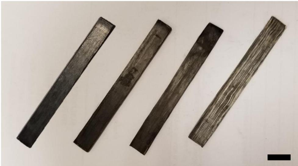
**Figure 4-5** Some of the flex bars used for 3-point bending testing (scale bar: 10 mm)
