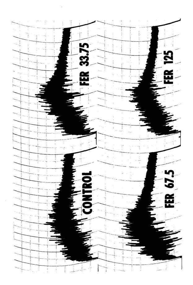
Fig. 7. Mixograms showing the combination of maleic acid (MA - 2000 ppm) with cysteine (20 ppm).
