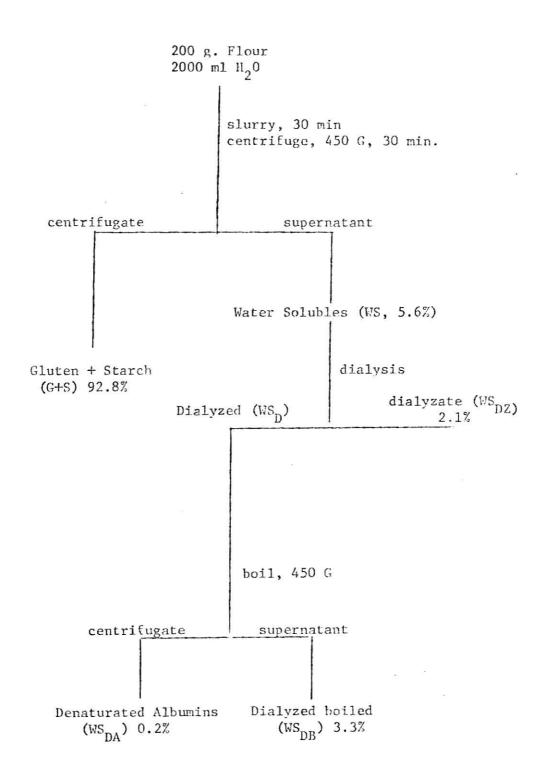
reduced to a powder in a mortar. Figure 1 illustrates the fractionation scheme and the fraction amounts recovered based on flour weight.
