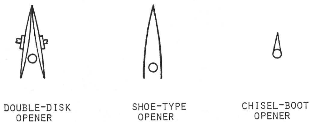
Figure 2. Methods Used for Furrow Opening and Seed Placement.
