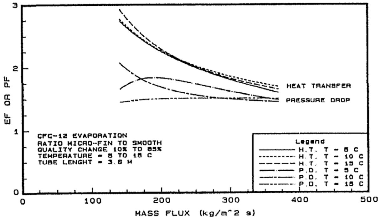
Figure 11 Heat transfer enhancement factor and pressure drop penalty factor for evaporation of CFC-12
