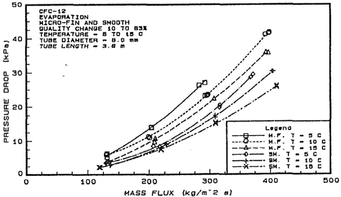
Figure 10 CFC-12 evaporation pressure drops in a smooth tube and micro-fin tube
