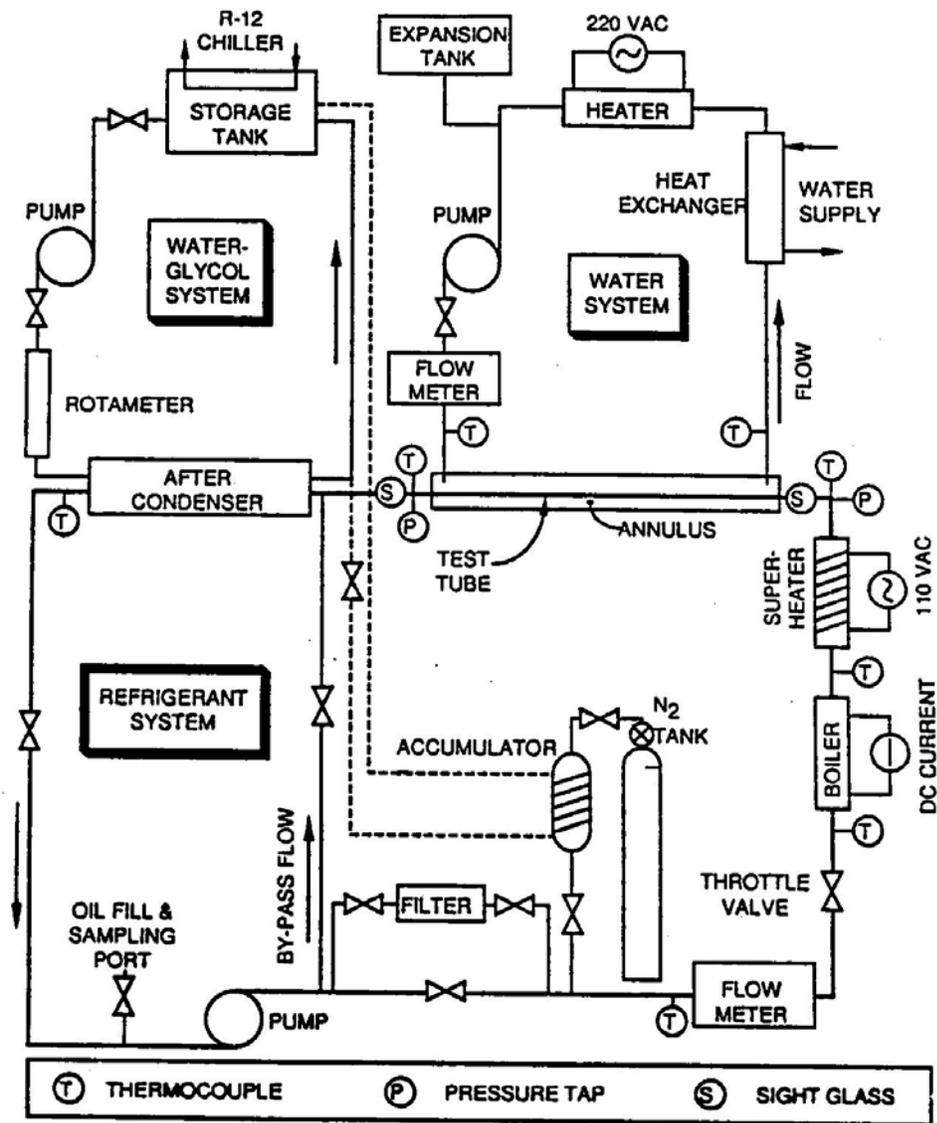
Figure 1 Schematic drawing of test facility
