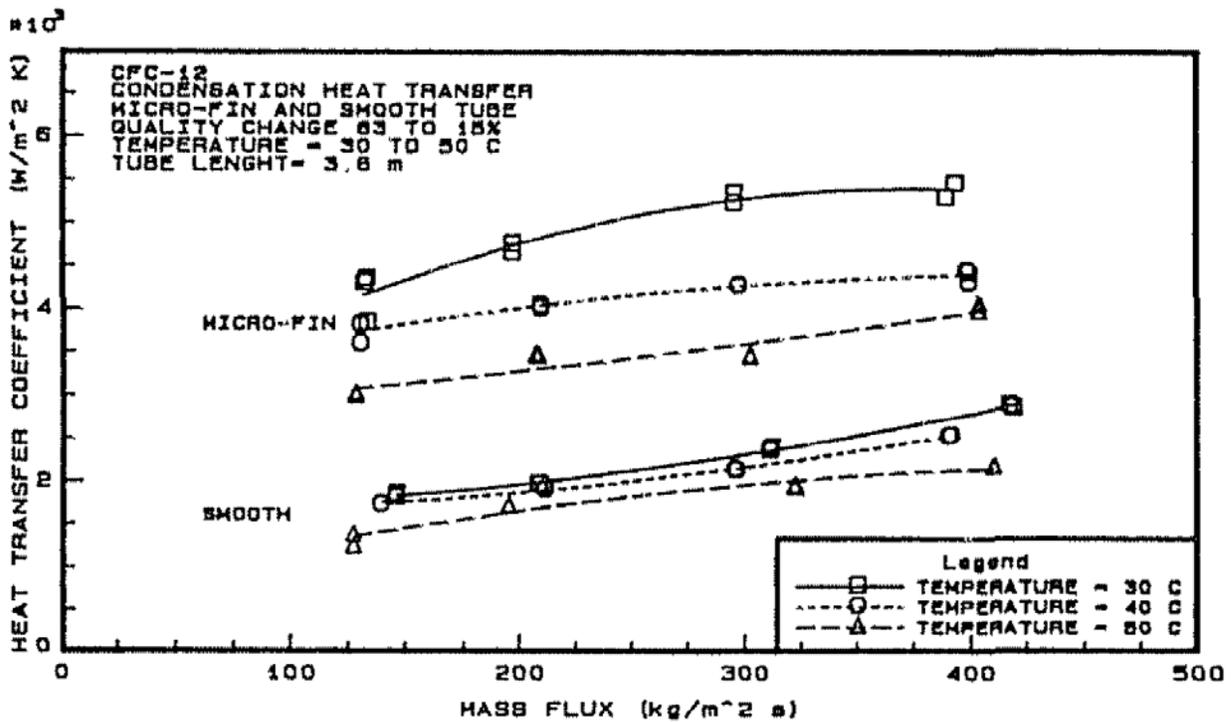
Figure 12: CFC-12 condensation heat transfer coefficients in a smooth tube and micro-fin tube
