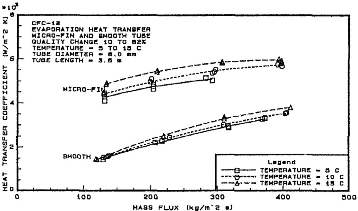
Figure 9 CFC-12 evaporation heat transfer coefficient in a smooth tube and micro-fin tube
