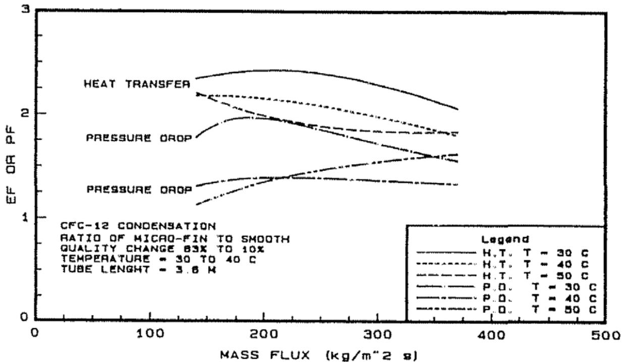
Figure 14 Heat Transfer enhancement factor and pressure drop penalty factor for condensation of CFC-12
