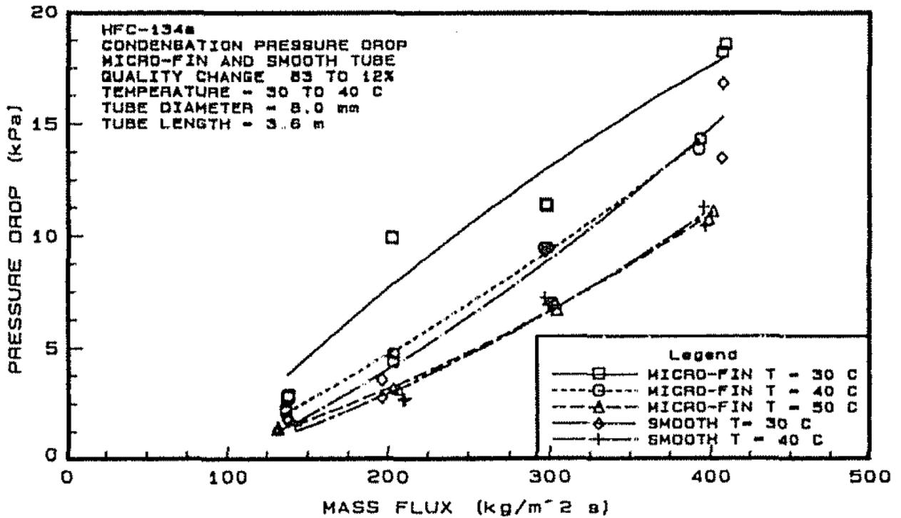
Figure 7 HFC-134a condensation pressure drops in a smooth tube and micro-fin tube.
