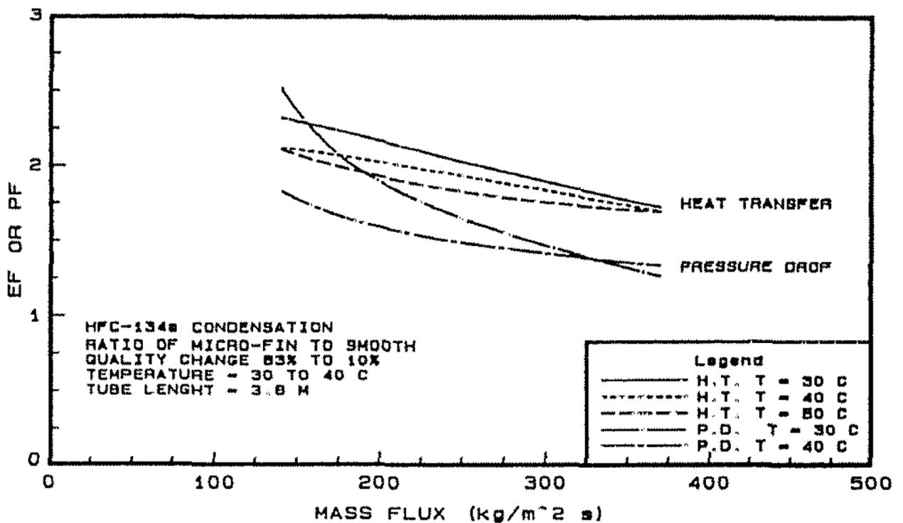
Figure 8 Heat transfer enhancement factor and pressure drop penalty factor for condensation of HFC-134a
