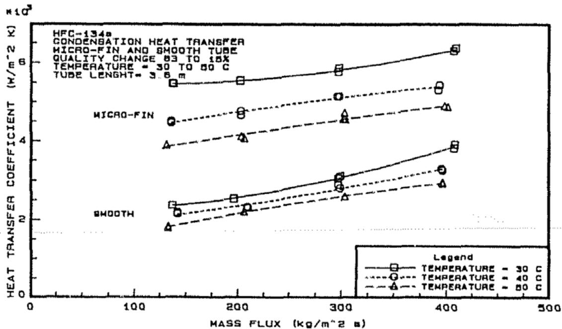
Figure 6 Condensation heat transfer coefficients in a smooth tube and micro-fin tube
