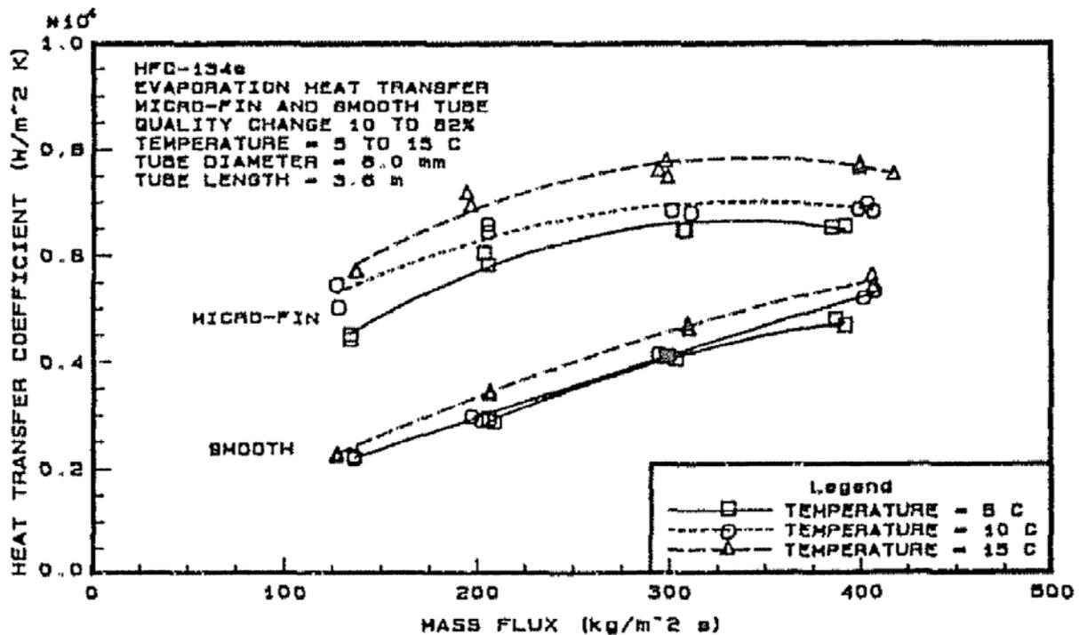
Figure 3: HFC-134a evaporation heat transfer coefficients in a smooth tube and micro-fin tube
