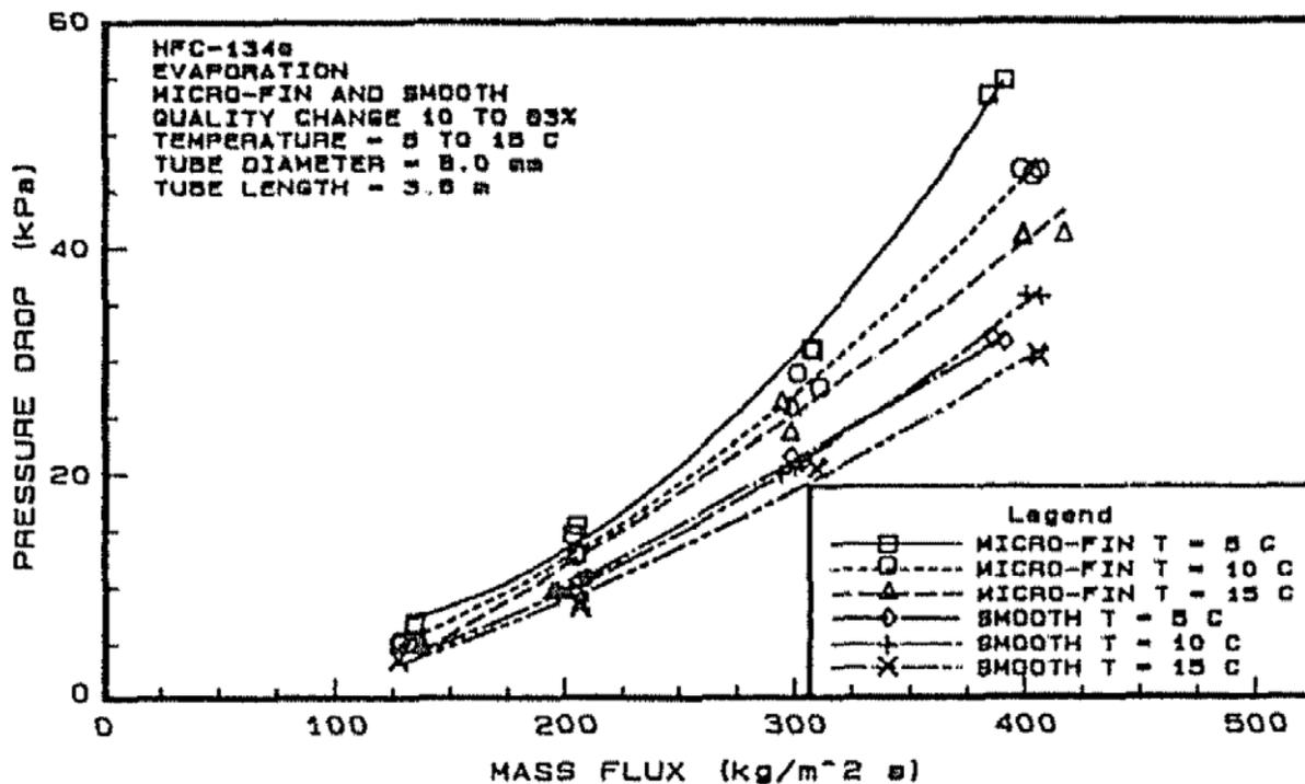
Figure 4: HFC-134a evaporation pressure drop in a smooth tube and micro-fin tube
