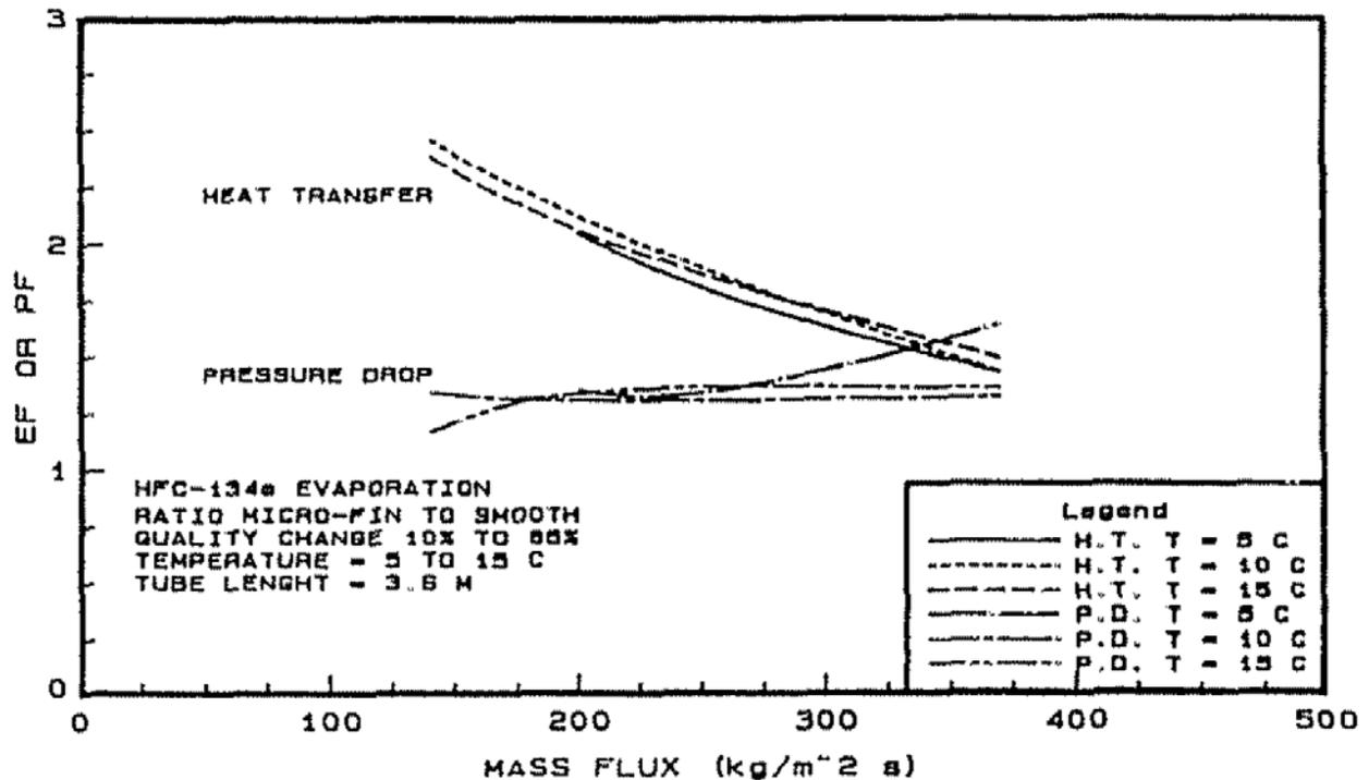
Figure 5: Heat Transfer enhancement factor and pressure drop penalty factor for evaporation of HFC-134a
