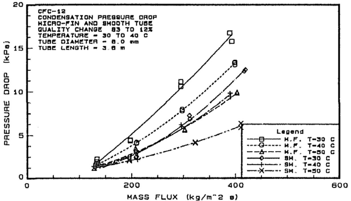
Figure 13 Condensation pressure drops in a smooth tube and micro-fin tube
