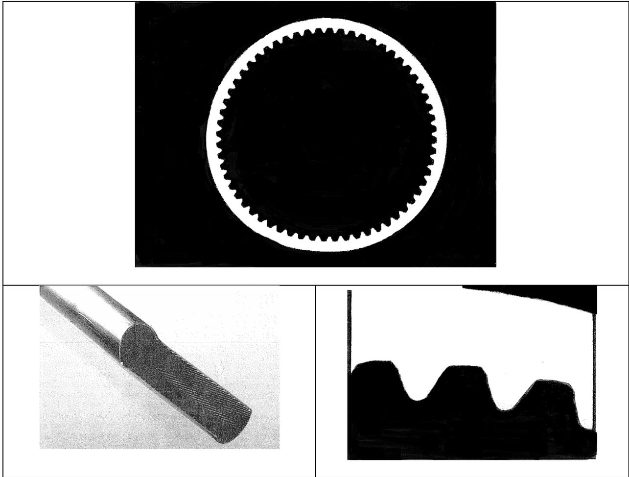
Figure 2 Photograph of the micro-fin tube
