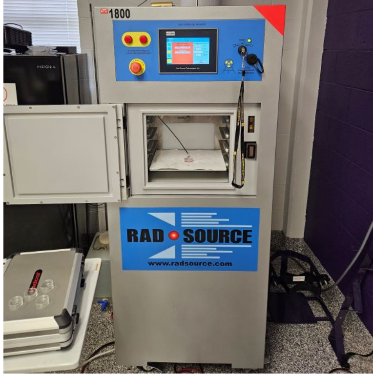
Figure 2.8: RadSource RS 1800 biological irradiator used as a source of x-rays.
