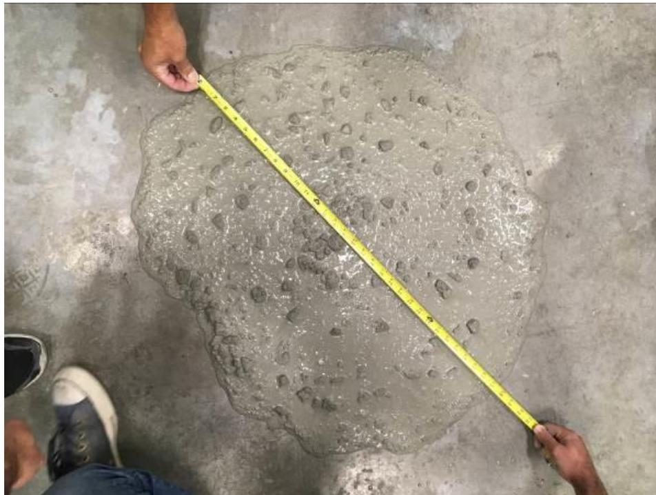
**Figure 63. Slump-flow (spread) of segregated mix (B161)**
