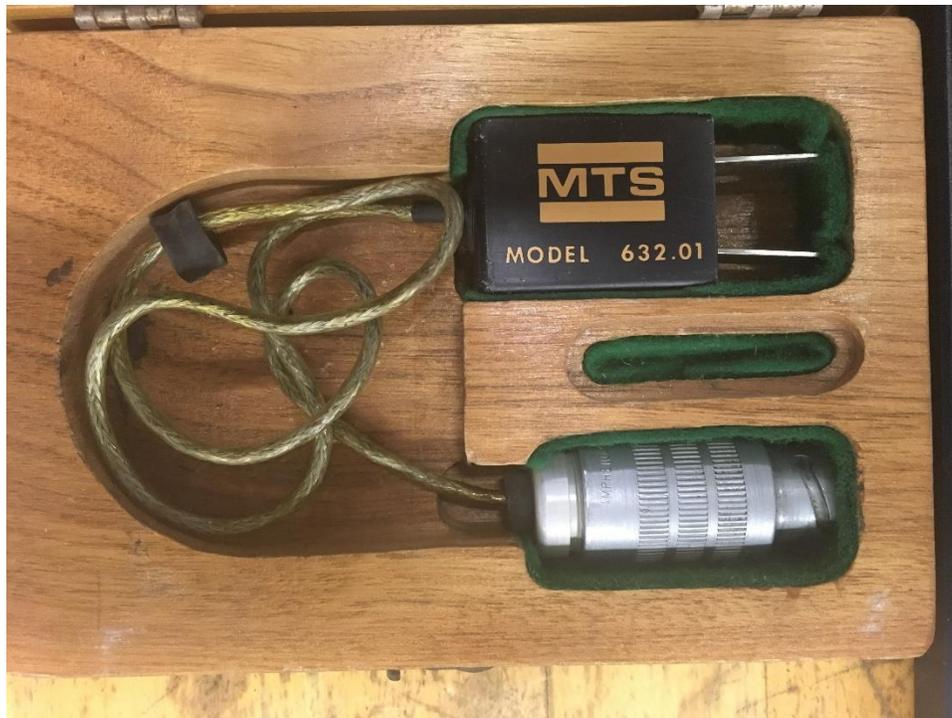
**Figure 17. Clip Gauge utilized in this study**
