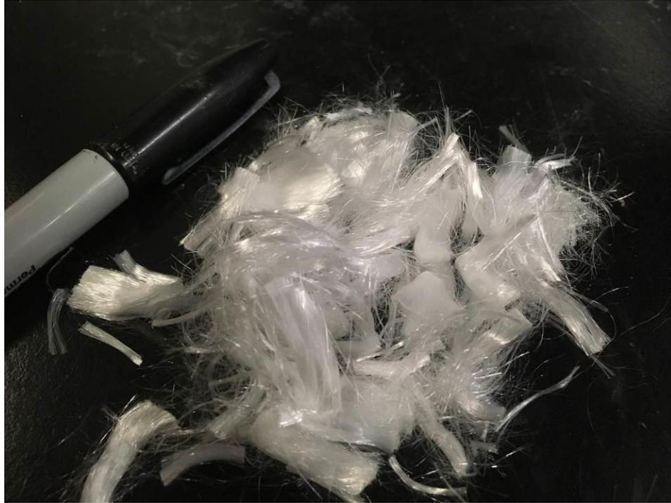
**Figure 73. Polymer Fiber**
