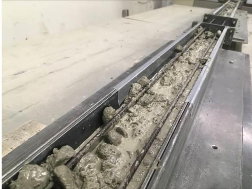
**Figure 64. Segregation of Mix B161 during casting**
