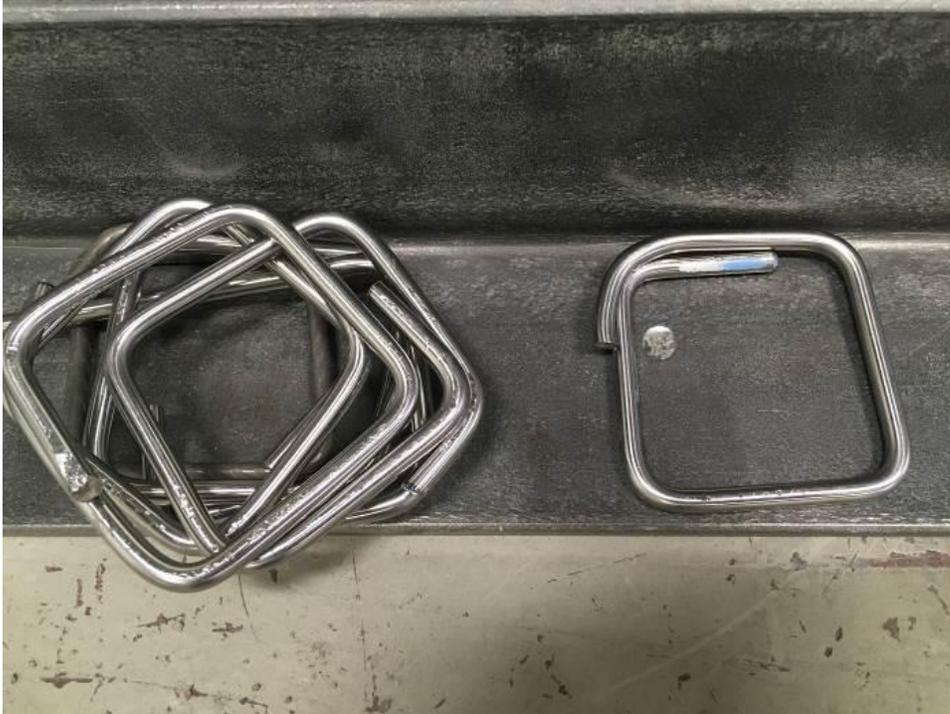
**Figure 82. Stirrups with 5 bends made at KSU lab**
