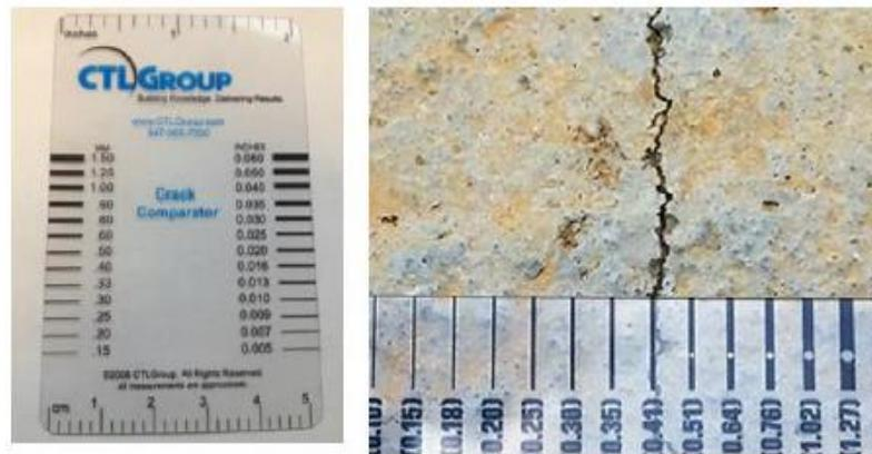
**Figure 59. Crack measurement through crack comparator**
