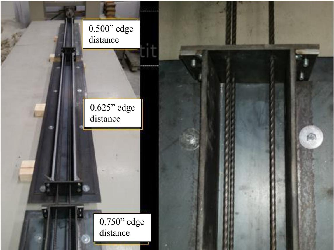
Figure 57. Prestressed prisms forms (Savic, Beck et al. 2018)
