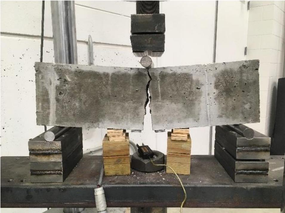
**Figure 21. Fatigue crack growth test set up.**
