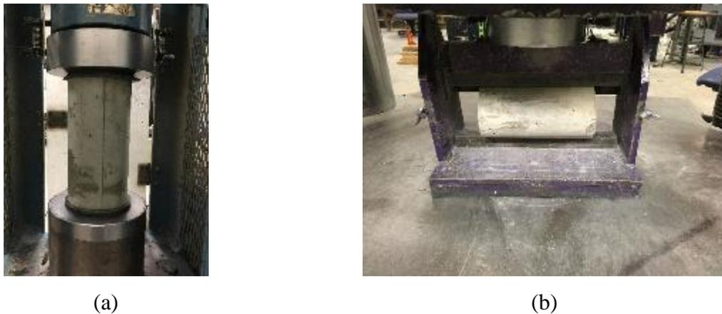
**Figure 15. a) Compressive strength test setup. b) Splitting tensile strength test setup**
