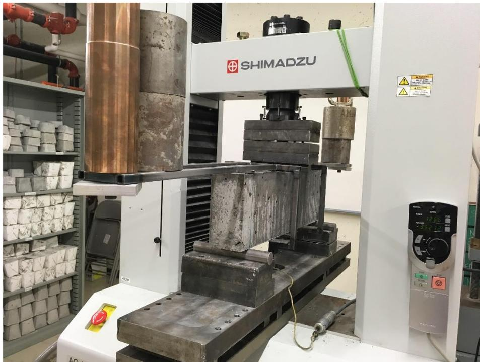
**Figure 18. Fracture toughness test setup**
