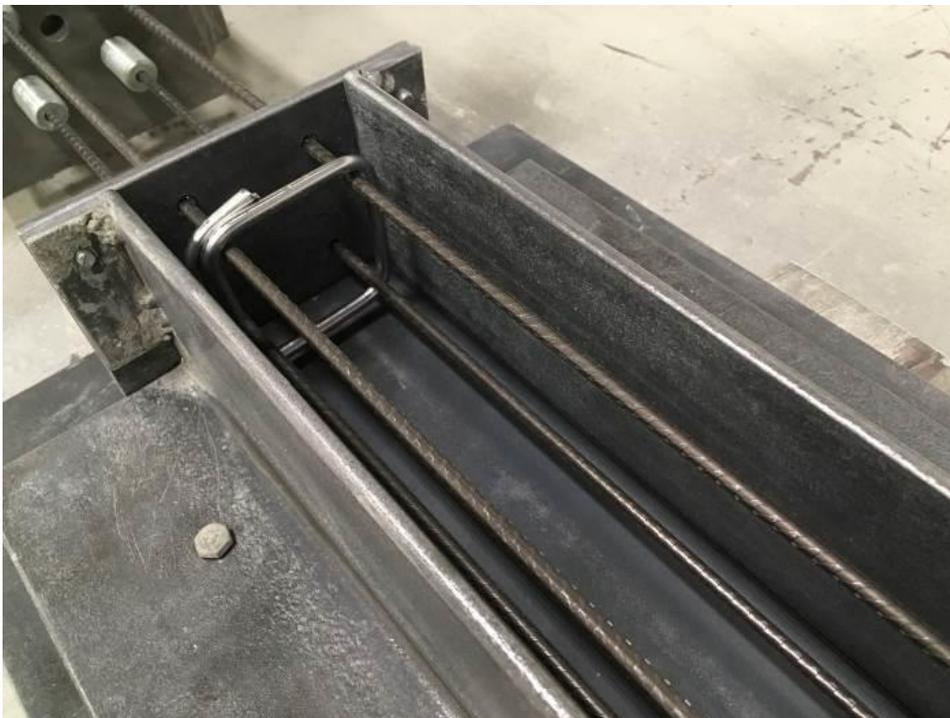
**Figure 83. Stirrups preparation and set up**
