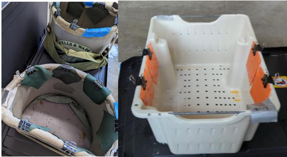
Figure 6.1. Nylon and HDPE coupons positioned SDC spray application.
