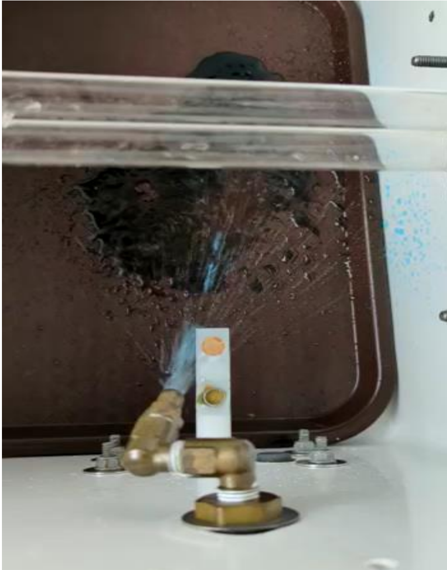
Figure 4.1. . Rod after removal from CDC biofilm reactor with 3 coupons inserted into spray application box.
