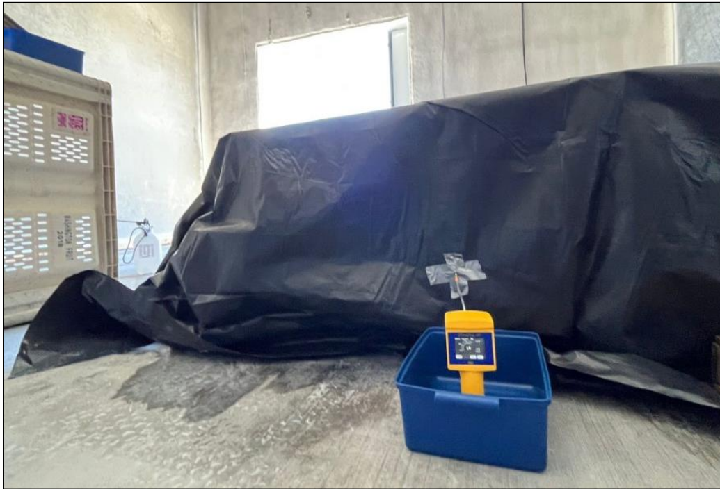
Figure 6.3. Bins covered with polyethylene vapor barrier for ClO 2 treatment.
