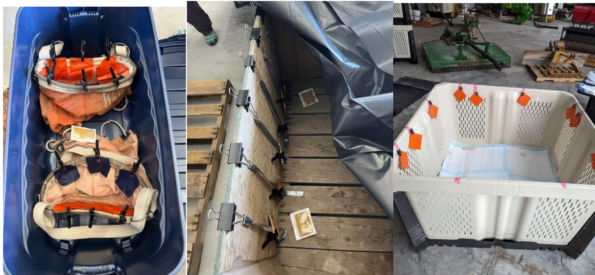
Figure 6.2. Nylon, wood, and HDPE coupons prepared for ClO 2 treatment.
