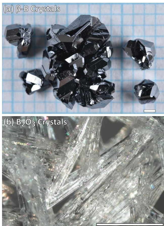
Figure 4-6. Images of (a) \beta -B and (b) B_2O_3 precipitated from a Cu-CuO-B flux. B_2O_3 crystals only precipitated from experiments that used high concentrations of oxygen. The scale bars are 1 mm.
