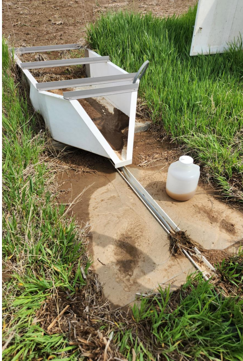
Figure 2 An image of a 0.45 m H-flume and sampling tube located at the plot outlets at the KAW
