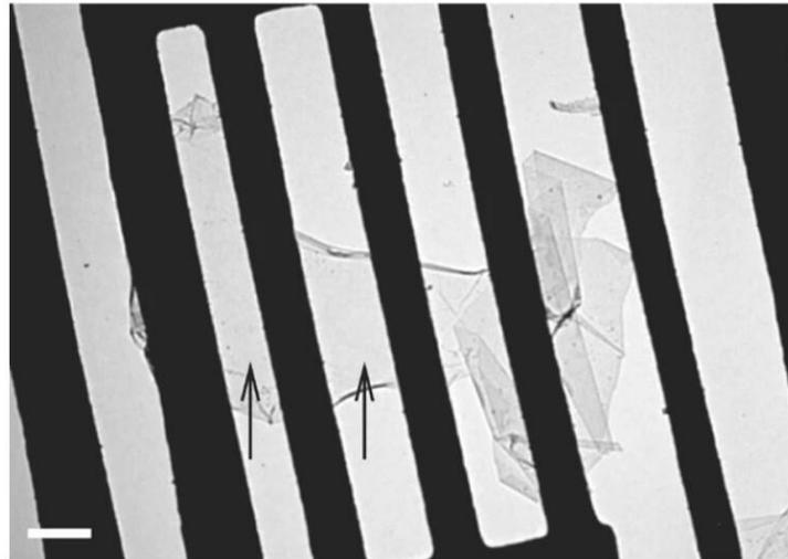
Figure 1.4. TEM image of micromechanical cleavage graphene film after electron-beam lithography and etching step. (reproduced with permission from Ref [23])
