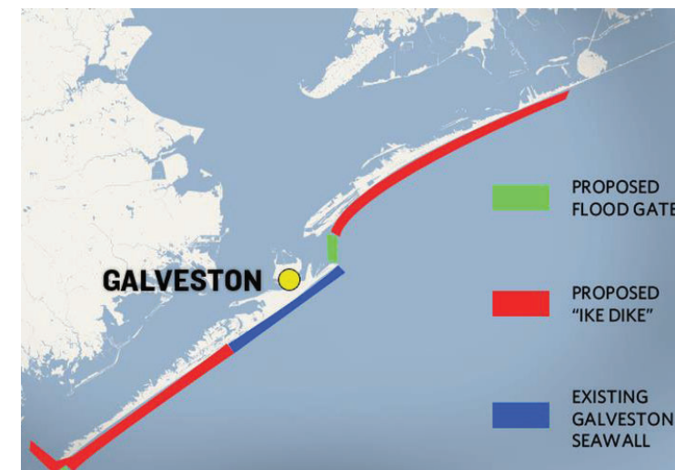
Figure 5.8: Location of the dike in dune and proposed floodgates (The Center for Beaches and Shores 2018)
