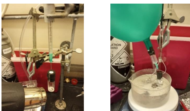
Figure E1: (Left) flame dried ZnCl 2 and LiCl under vacuum by heat gun (Right) dropwise addition of Grignard to ZnCl 2 and LiCl in THF under N 2 balloon.
