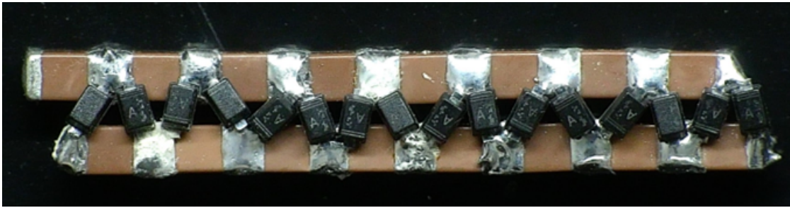
Figure 3.3: An eight stage CW hybrid ladder makes up half of the total 16 stage CW ladder required to run the PMT.
