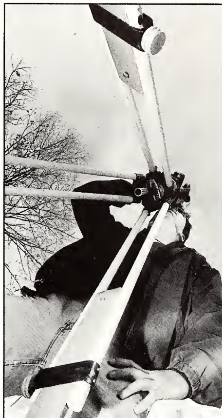
William Marsh, senior in civil engineering, sights an elevation through a theodolite east of Kedzie Hall. Marsh, along with Matt Janzen, junior in environmental design and Bob Atkins, senior in construction science, produced a topographic map of Kedzie. (Photo by J. Kyle Wyatt)
