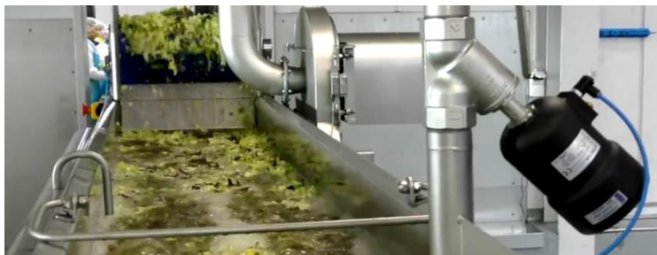
Figure 1.5A. Leafy greens going through flume washing. Retrieved from Sormac (2020).
