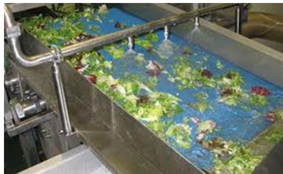
Figure 1.5A. Leafy greens going through flume washing. Retrieved from Sormac (2020).
