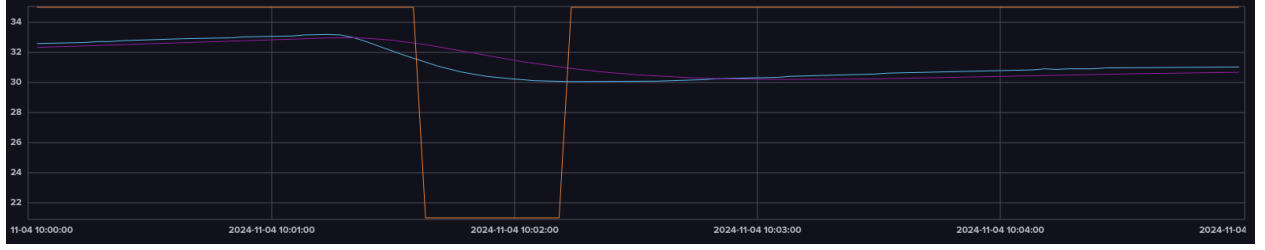
Figure 4.1: Graph of the recorded temperature (blue), predicted temperature (purple) and target temperature (yellow) of Inc-RH during a lid open event
