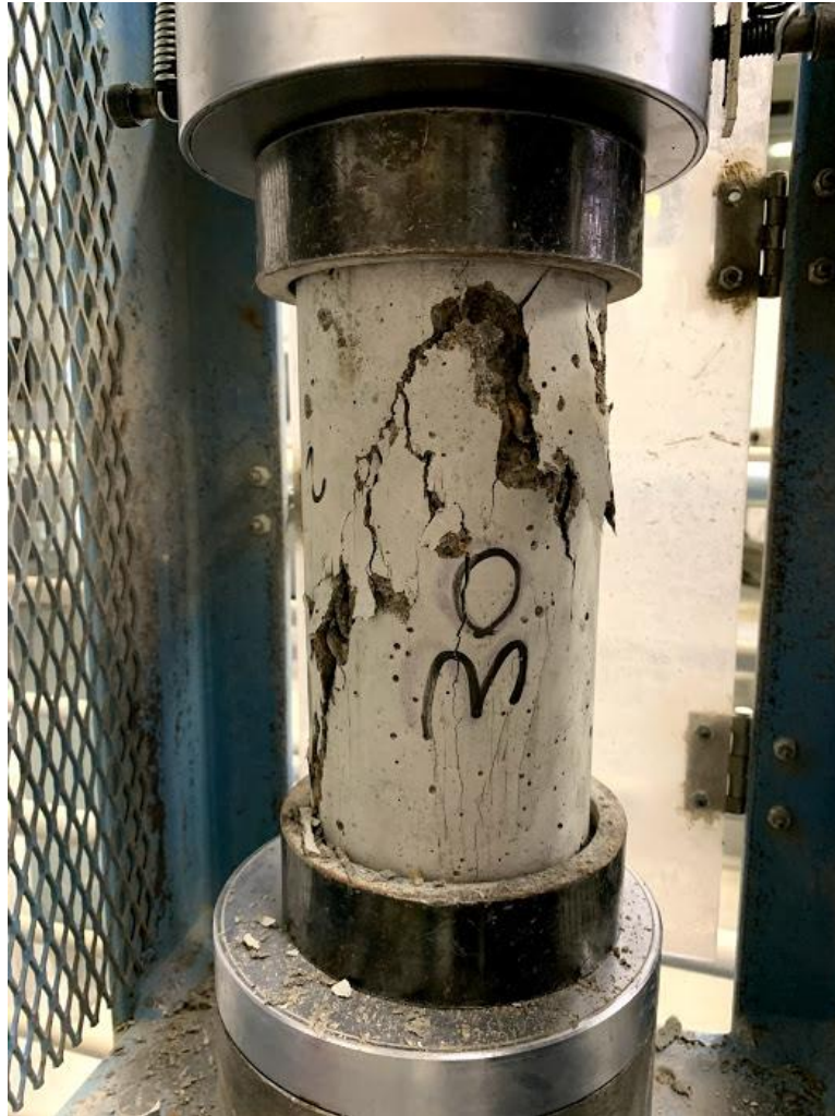
Figure 3-5 Cracked Cylinder - Compression Test
