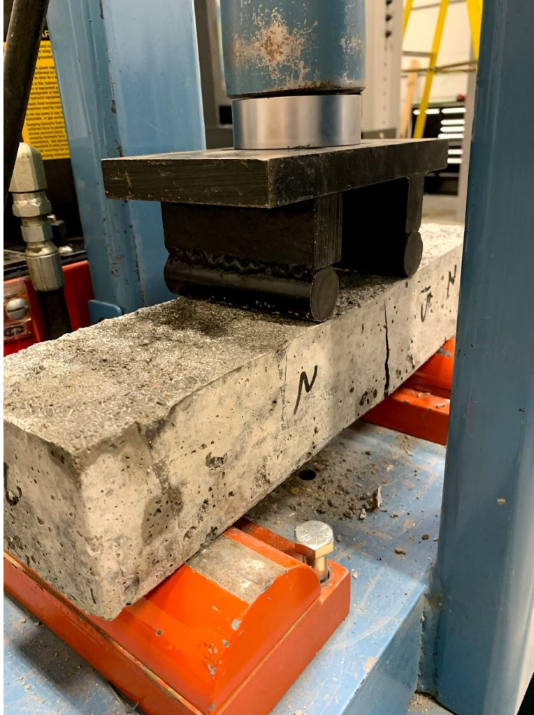
Figure 3-9 Cracked Prism - Modulus of Rupture
