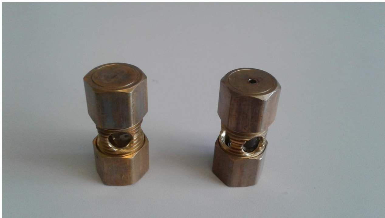
Figure 2.3: Picture indicating how reaction vials were placed into brass vessels for heating.
