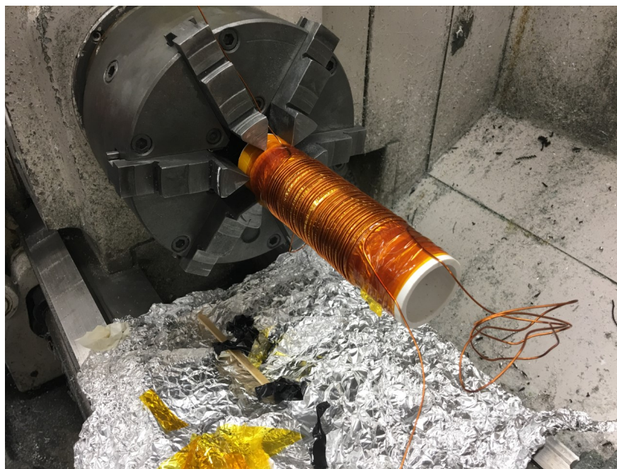
Figure 4.8: A photograph of the main coil of the RF oscillator during winding. The secondary coil has been wound underneath and the primary coil is shown after epoxy has been applied. The next step is a layer of Mylar to keep the coils from shorting together. Following Mylar, the final step is the winding of the feedback coil
