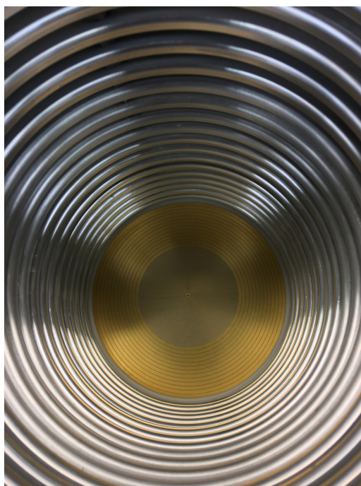
Figure 4.13: Inside the rings of the gas stopping cell showing the RF carpet that is used to initially concentrate all positively-charged ions from the decay of ^{233}\text{U} into a beam.
