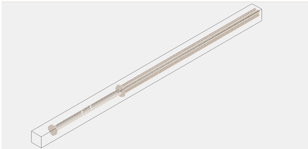
Figure 4.2: The SIMION geometry used to model the trajectory of the ^{229}\text{Th}^{3+} ions. Starting from the right, shown is the first radiofrequency quadrupole (RFQ), mass separation quadrupole (QMS), second RFQ, orifice place, ion trap, and the microchannel plate (MCP) detector.
