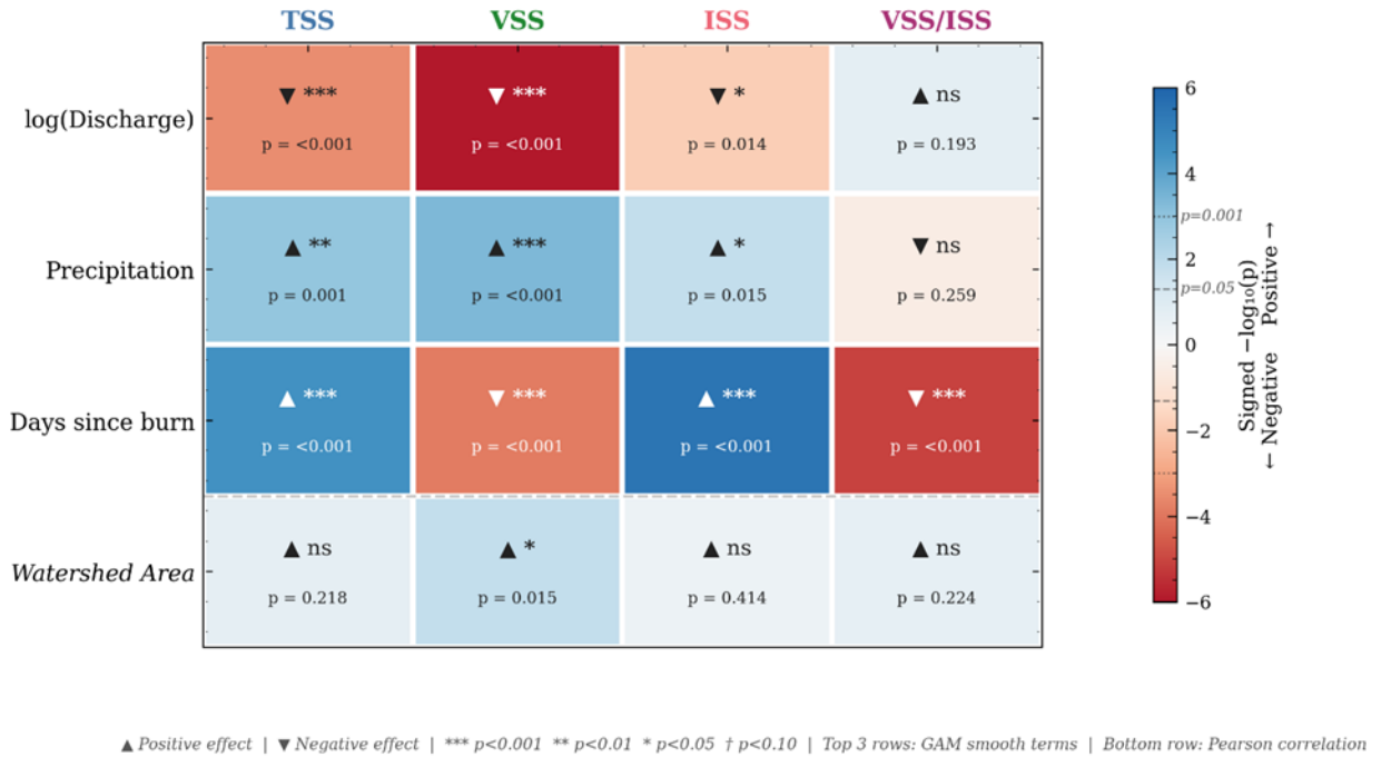
Figure 4.4: Divergent environmental controls on organic versus inorganic suspended sediment fractions revealed by generalized additive model (GAM) analysis. Heatmap of signed \log_{10}(p\text{-value}) for each predictor (rows: log discharge, precipitation, days since burn, watershed area) across four response variables (columns: TSS, VSS, ISS, VSS/ISS ratio). Blue shading indicates significant positive effects; red shading indicates significant negative effects; color intensity is proportional to statistical significance. Upward triangles denote positive effects; downward triangles denote negative effects.
