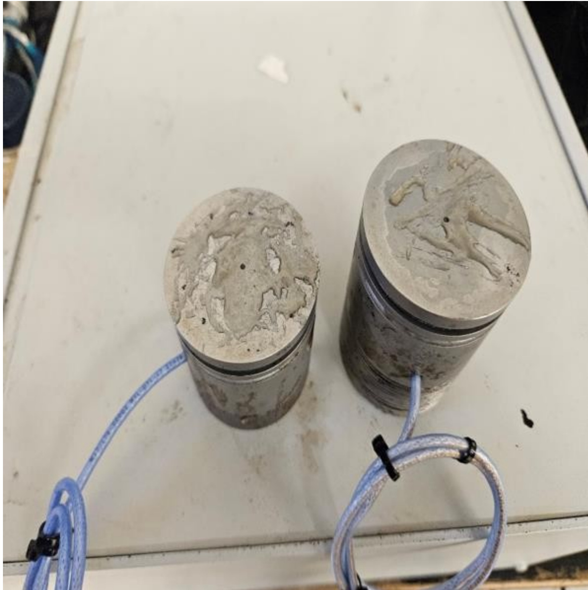
Figure 2.2. Core plugs mounted between NX-size piezoelectric platens and transducers prior to loading. Honey couplant is applied to the sample faces to ensure acoustic coupling between the platens and the rock. Adapted from (King, 2025).
