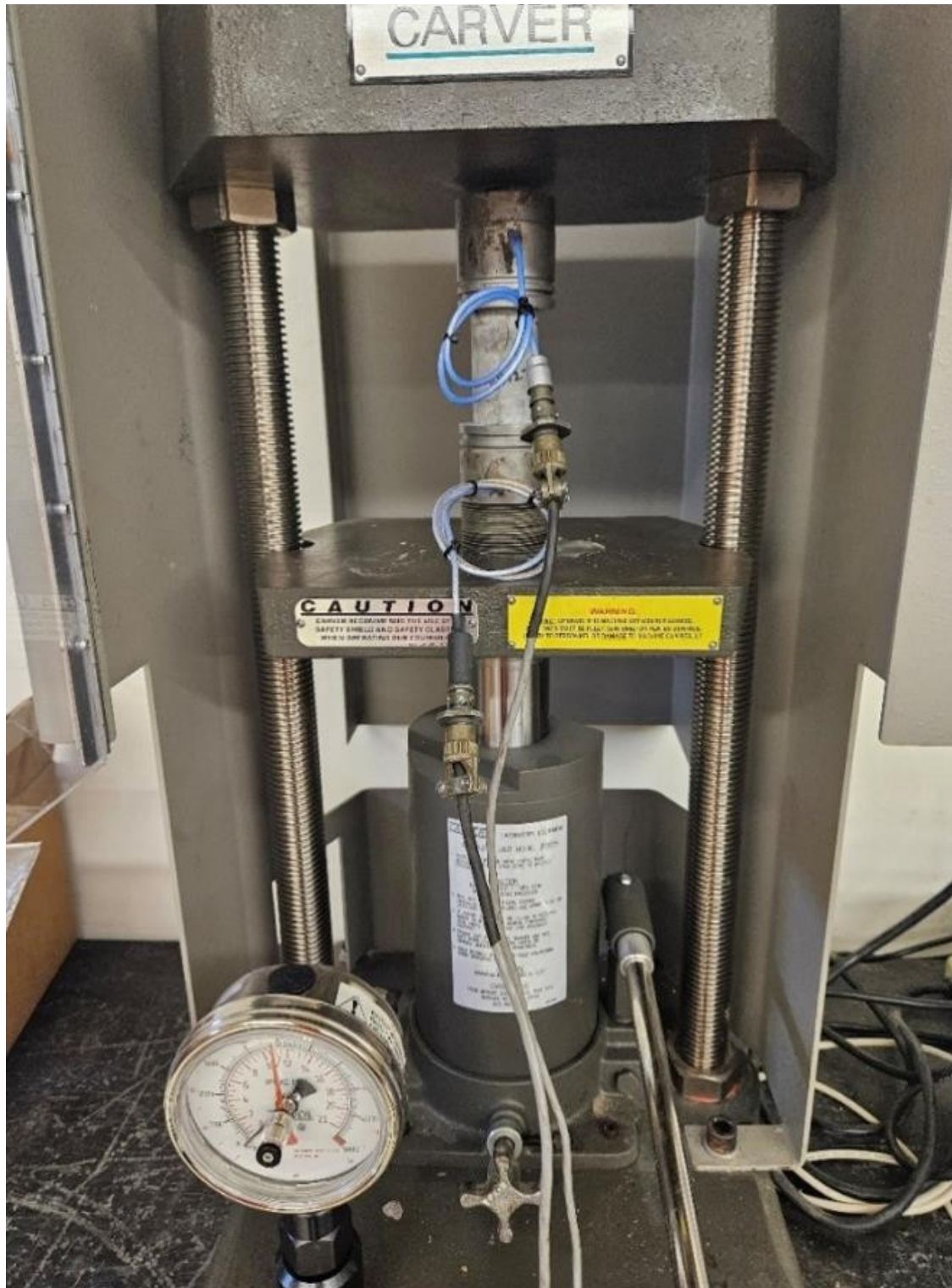
Figure 2.1. Carver hydraulic press with GCTS ULT-100 ultrasonic velocity test assembly. The press provides uniaxial confining stress to the core plug mounted between piezoelectric platens within the central loading frame. Adapted from (King, 2025).
