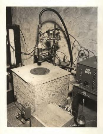
have enabled variations of velocity at any radial position to be compared to the exit velocity at the nozzle. Plate VIII shows this arrangement of equipment.
