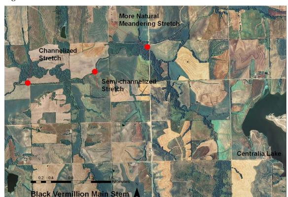
Figure 4.10 Natural meanders to channelized reaches on Main Stem 2006 aerial.
