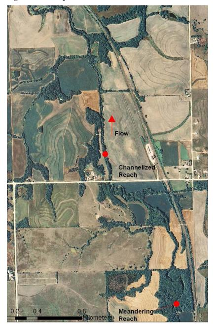
Figure 4.7 Example of channelization and natural meander bends in Irish Creek.
