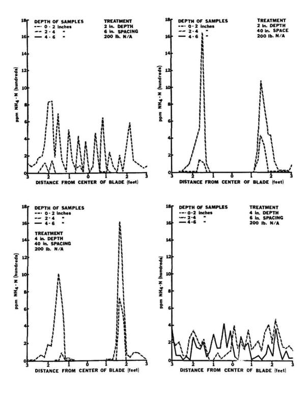
2-inch application depth produced a similar pattern. Ammonia concentrations at the release points exceeded 1000 ppm and one approached 1600 ppm NH<sub>4</sub><sup>+</sup>-N. Total lateral movement was about 18 inches. The 40-inch spacing at this 200 lb rate could provide an adequate distribution of nitrogen for crop growth on this sandy soil. The 6-inch spacing, however, yielded an excellent distribution of ammonia across the entire width of the blade.
