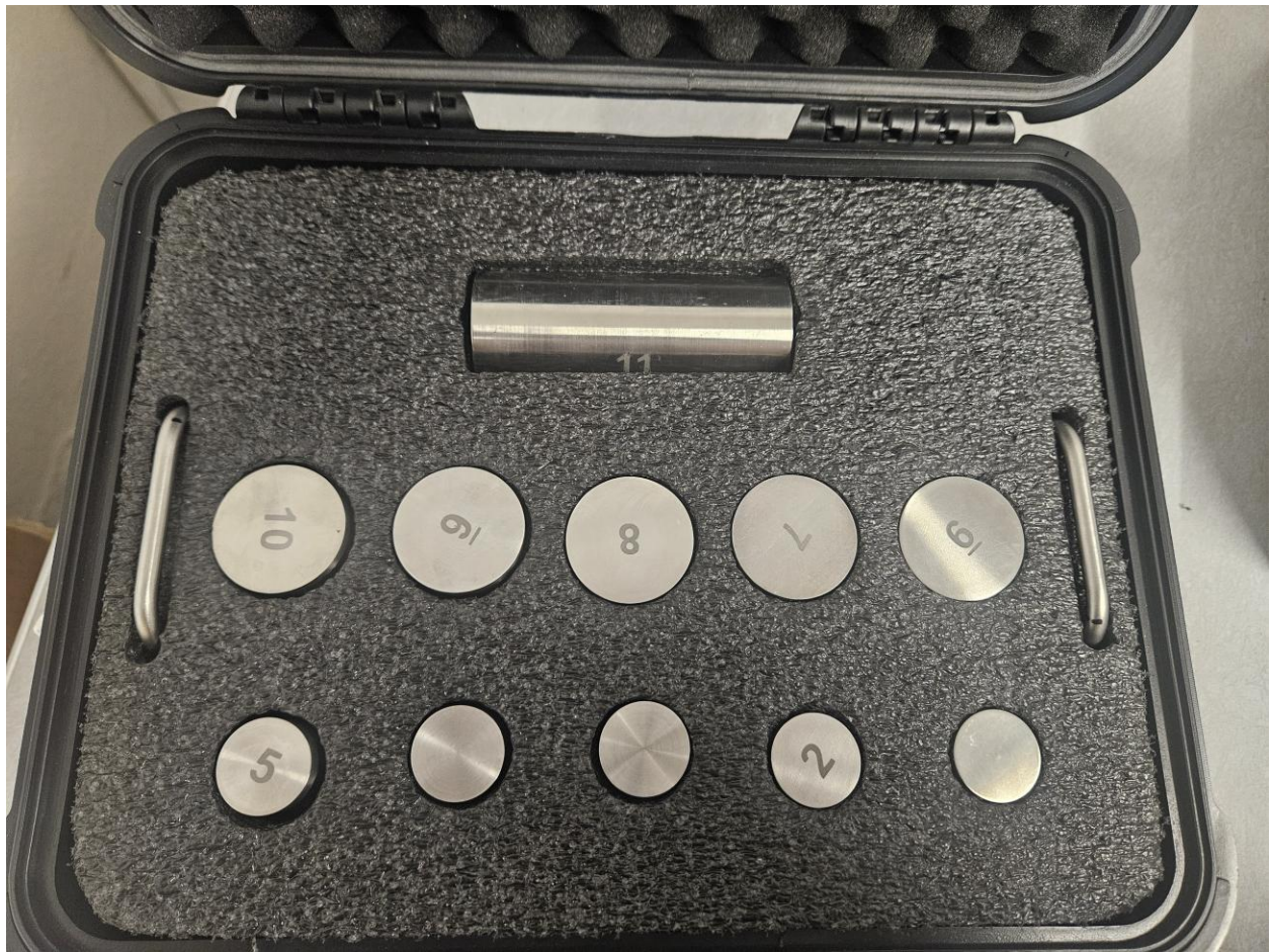
Figure 3.11 Spacers used in porosimeter.
