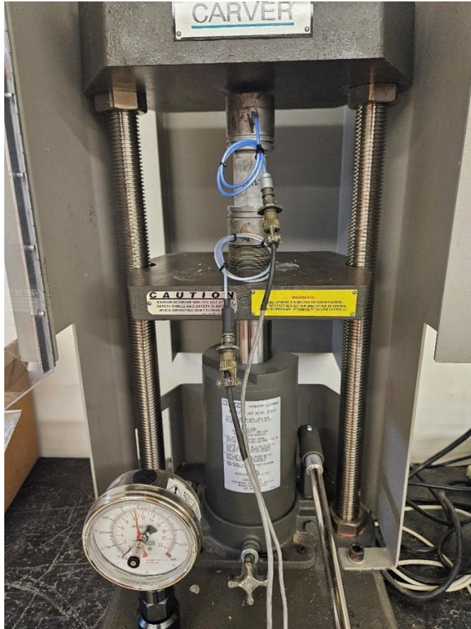
Figure 3.2 Carver hydraulic press that exerts pressure.
