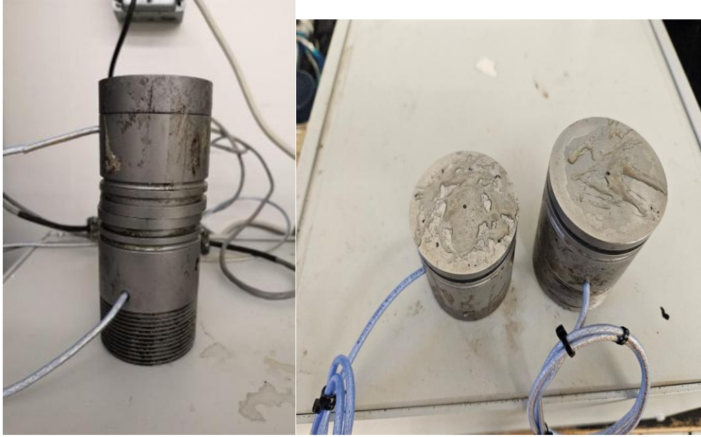
Figure 3.5 Face to face of platens (left). Honey used on platens to ensure good coupling (right).
