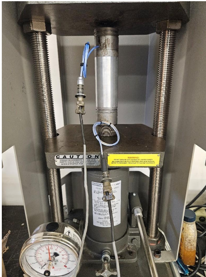
Figure 3.6 Velocity measurements being taken on aluminum core.
