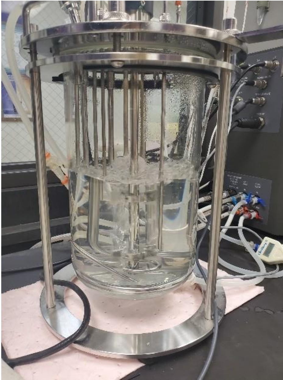
Figure 2.1. A photograph of the bioreactor in operation with air injection and agitation
