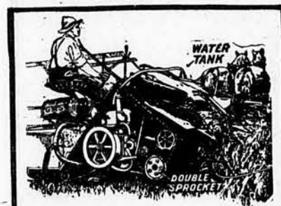
This shows how the same 4 h. p. engine may be attached to rear of binder. It saves two horses on 8-foot binder, and in a wet season it saves the crop, as it makes it possible to cut even when the bull-wheel slips. Also used on potato diggers, corn binders, etc.
